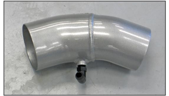
19. Install the provided 90° vent fitting into the K&N® intake tube as shown.
