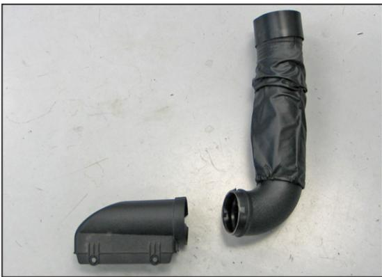
11. Remove the fresh air duct from the fresh air scoop.
