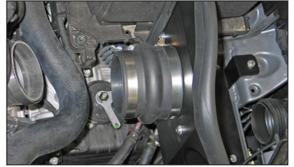
18. Install the provided hump hose (5-576) onto the filter adapter and secure with the provided hose clamp.
