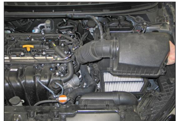
6. Remove the upper air box/intake hose assembly from the vehicle.
