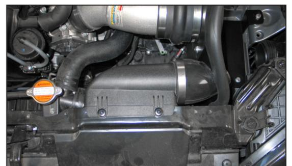
22. Install the fresh air intake scoop assembly so the silicone hose passes through the hole in the heat shield, then secure with the factory retaining clips.
