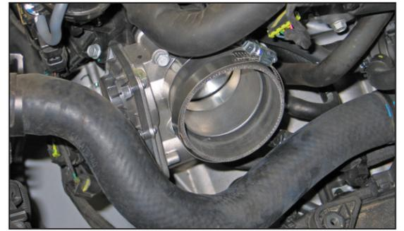
17. Install the provided silicone hose (084036) onto the throttle body and secure with the provided hose clamp.
