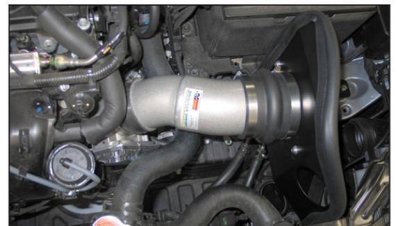
20. Install the K&N® intake tube into the silicone hump hose and then into the silicone hose attached to the throttle body. Secure with the provided hardware.
