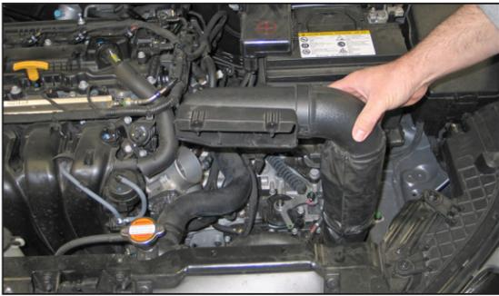
10. Remove the fresh air intake duct from the vehicle.
