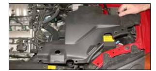
10. Remove the battery cover, which is secured by 4 plastic rivets and one bolt as shown.
