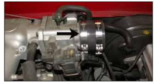
17. Install the silicone hose and hose clamps onto the throttle body and secure as shown.
