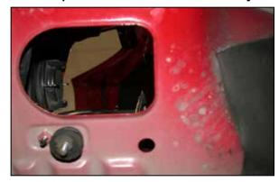
26. From underneath the vehicle, install the rubber mounted stud onto the existing stud located on the bottom of the inner fender rail as shown.
