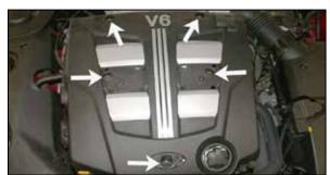
3. Remove the engine cover, which is secured by 5 bolts as shown
