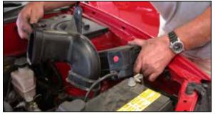
16. Remove the fuse box bolts, lift upward, then, remove the air cleaner duct as shown.
