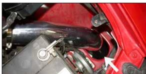
27. Slide the cold air tube through the fender from underneath the vehicle and into the silicone hump hose as shown.
