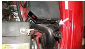
14. Remove the bolt that secures the air cleaner duct to the inner fender as shown.
