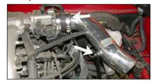
21. Slide the intake tube into the silicone hose on the throttle body, then line up the threaded boss with the bracket from step 19 and secure with the provided hardware, but do not tighten at this time.
