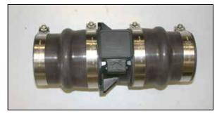
24. Install the two silicone hump hoses and hose clamps onto the mass air sensor and secure as shown.
