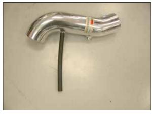
20. Install the provided hose onto the K&N $^{\mbox{\tiny 6}}$  intake tube as shown.
