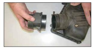
23. Remove the mass air sensor from the air cleaner cover as shown.
