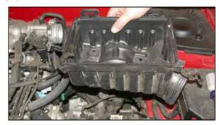
9. Remove the lower air cleaner assembly, which is secured by three bolts.
