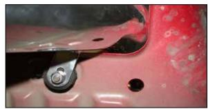
28. Line up the cold air tube bracket with the rubber mounted stud from step 26 and secure with the provided hardware as shown.
