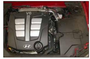
37. Reinstall the engine cover as shown.
