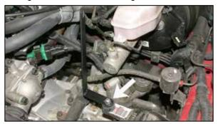
19. Install the provided bracket onto the rubber mounted stud and secure using the provided hardware, but do not tighten completely at this time.
