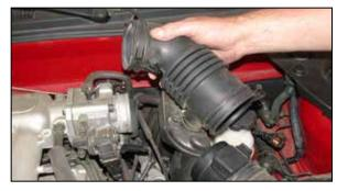
7. Loosen the hose clamps at the throttle body and at the mass air sensor, then, remove the stock intake tube as shown.
