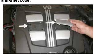
2. Remove the three engine cover panels using a flat blade screwdriver.
