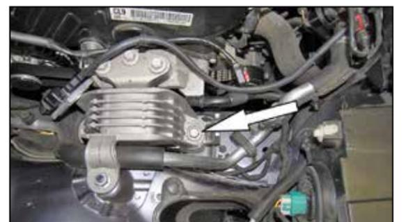
6. Remove the motor mount bolt show.
