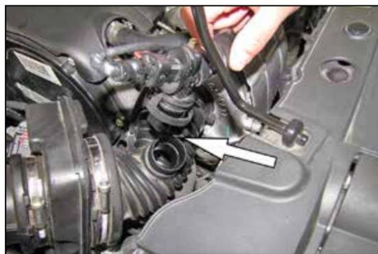
3. Release the locking tabs and then disconnect the pressure sensor from the factory intake tube.
