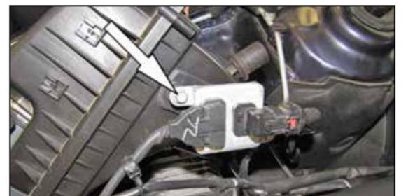
5. Lift up the air filter assembly to gain access to the electrical box attached to the air filter housing. Then remove the two bolts that secure the electrical box and separate it from the air filter housing and then remove the air filter assembly from the vehicle.
