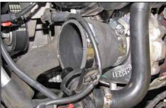
11. Install the provided step coupler (08713) onto the turbo inlet and secure with the provided hose clamp.
