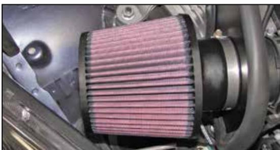
18. Install the K&N® air filter and secure it with the provided hose clamp.
