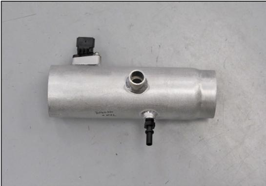
13. Install the provided NPT quick disconnect fitting into the K&N® intake tube as shown.
