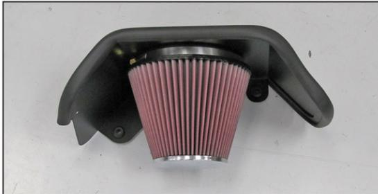
17. Install the air filter onto the filter adapter and secure with the provided hose clamp.
