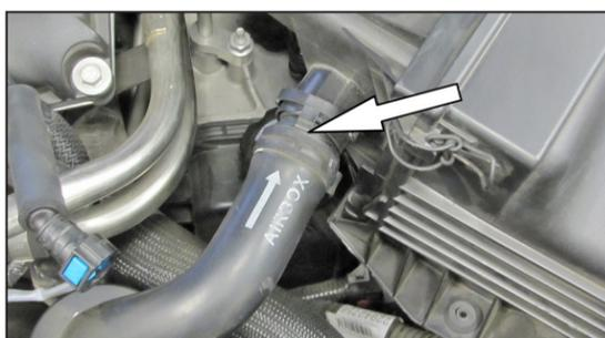
6. On vehicles equipped with air injection, disconnect the air injection hose at the quick disconnect fitting as shown.
