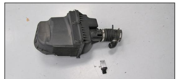
9. Remove the two screws securing the mass air sensor and then remove the sensor from the air box.
