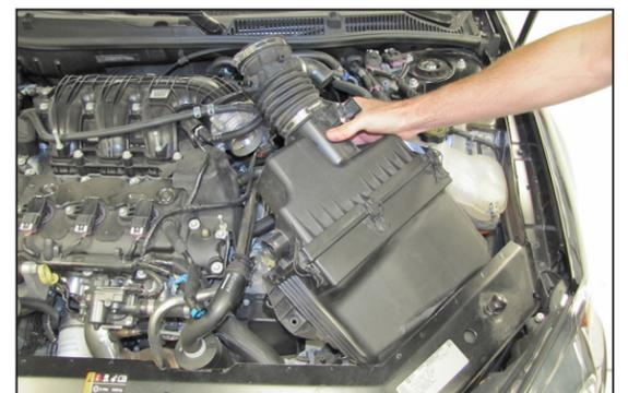
7. Lift up and remove the complete intake system as shown.
