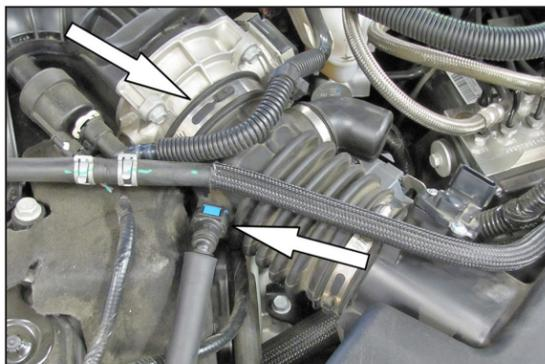
5. Loosen the hose clamp securing the factory intake tube to the throttle body, and then disconnect the crank case vent hose from the intake tube.
