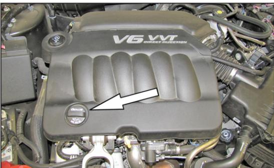
2. Remove the oil fill cap and then remove the engine cover from the engine. Reinstall the oil fill cap.
