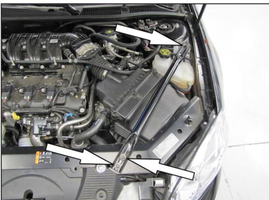
3. Remove the three bolts securing the body brace and then remove the body brace.
