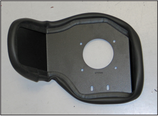
13. Install the provided edge trim onto the heat shield as shown. NOTE: Some trimming of the edge trim will be necessary.
