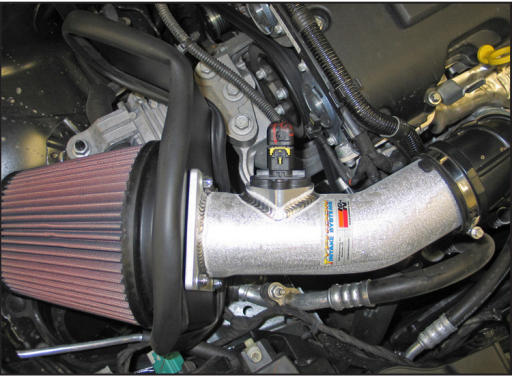
18. Connect the mass air sensor electrical connection.
