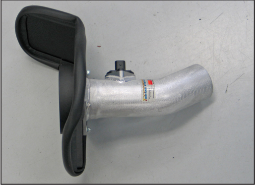
14. Assemble the tube, heat shield and filter adapter along with a gasket on each side of the heat shield, and secure with the provided hardware.
