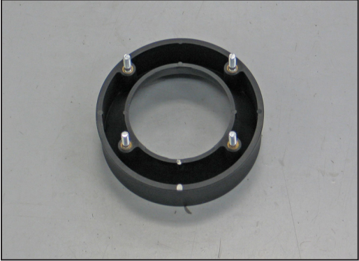
12. Install the four provided 6mm studs into the filter adapter as shown.
