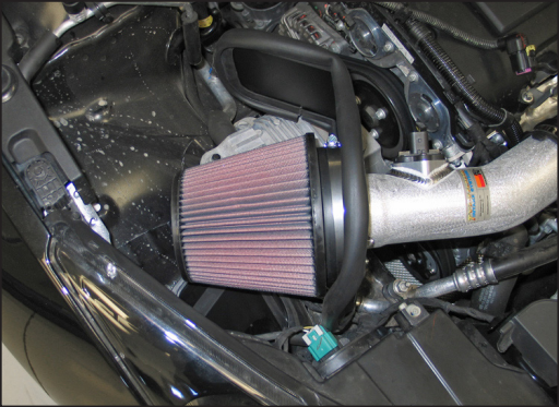
17. Install the K&N® air filter onto the filter adapter and secure with the provided hose clamp.
