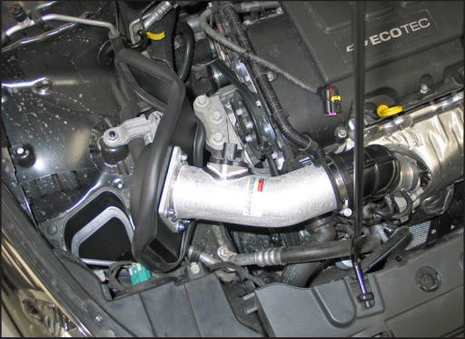
16. Install the intake assembly into the factory intake elbow and align the heat shield with the rubber mounted studs installed onto the mounting bracket. Align the intake for proper fit and secure with the hardware provided and factory hose clamps.
