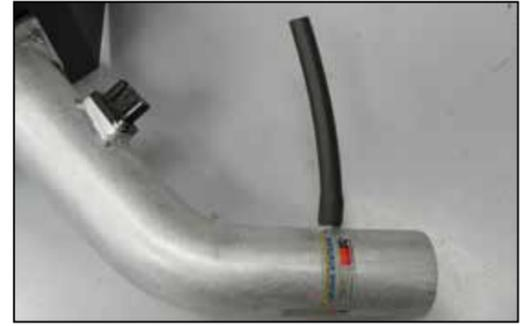
20. Install the provided crankcase vent hose onto the K&N® intake tube as shown.
