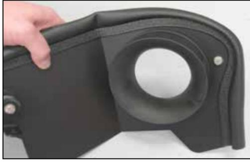
15. Apply one of the supplied gaskets to the filter adapter studs and then pass the studs through holes in the heat shield to install the filter adapter as shown.
