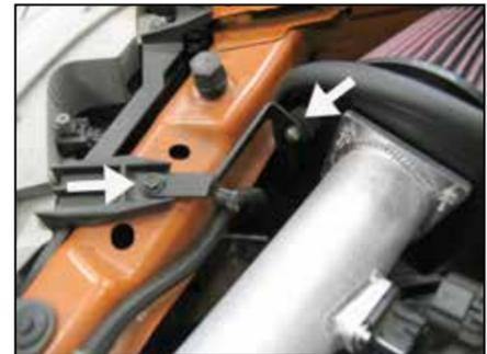
23. Install the "Z" bracket onto the headlight mounting bracket and rubber mounted stud as shown. Secure with the factory bolt removed in step #22 and the provided hardware.
