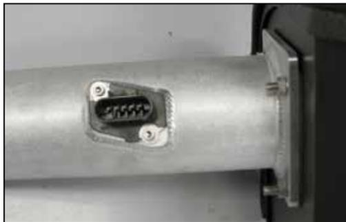
18. Install the mass air sensor into the K&N® intake tube and secure with the provided bolts.
