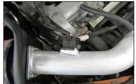
25. Reconnect the mass air sensor electrical connection.
