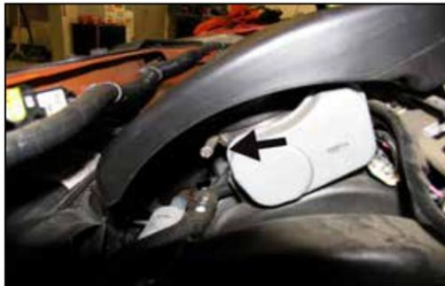
5. Loosen the hose clamp which secures the plenum to the throttle body.
