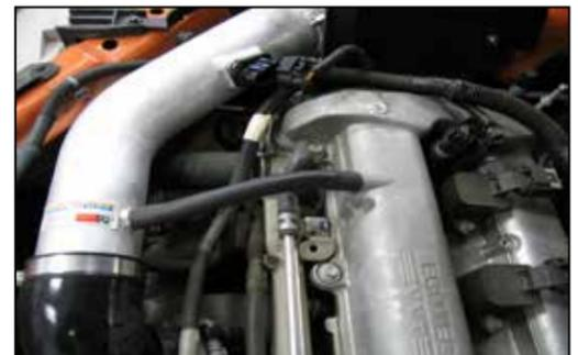
24. Install the crankcase vent hose onto the vent fitting on the valve cover.
