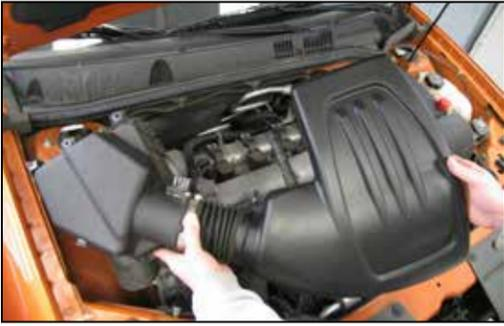
8. Lift the intake tract assembly off of the throttle body and then remove the complete assembly from the vehicle.
