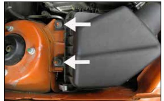
7. Remove the two nuts which secure the airbox to the inner fender.
