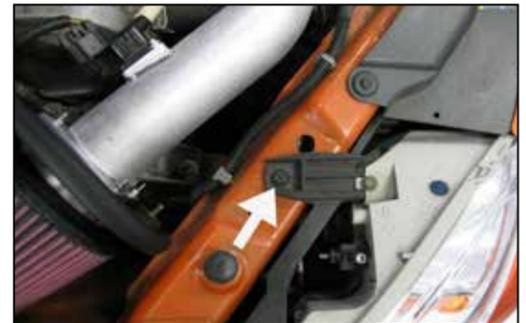
22. Remove the headlight mounting bracket bolt shown.
