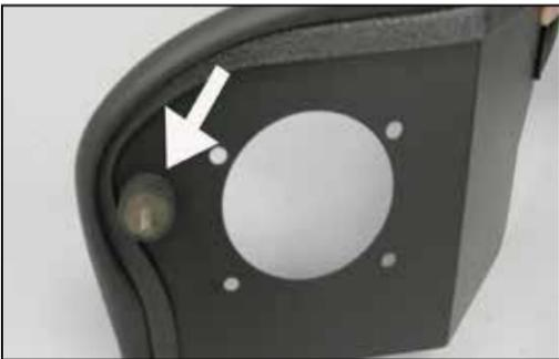
12. Install one of the supplied rubber mounted stud onto the heat shield as shown and secure with the provided hardware.
