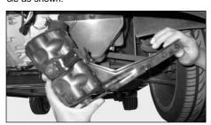
11. Remove the resonator box from the vehicle as shown.
