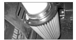
19. Fit the filter onto the "B" tube using the #44 hose clamp supplied.
