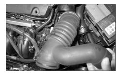
5. Unclip and remove the intake hose from the resonator box as shown.
