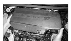
8. Unclip and remove the complete air box from the vehicle as shown.
