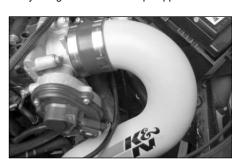
15. Fit the "A" tube into the sleeve using a #44 hose clamp. Do not fully tighten at this moment. NOTE: Before installing clean the inside of the 2 tubes with water and towel.
