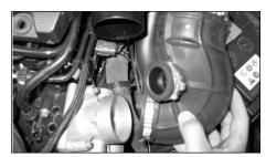
4. Unclip and remove the intake hose from between the air box and throttle body as
