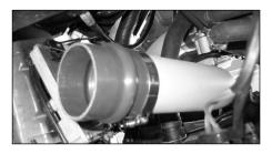
16. Fit the hump hose onto the "A" tube using a #44 hose clamp supplied.
