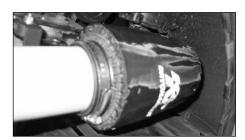
20. Fit the dry-charger onto the filter as shown. **NOTE:** The Drycharger's water repellant properties will last up to two years. See the parts list to re-order Drycharger if necessary.
