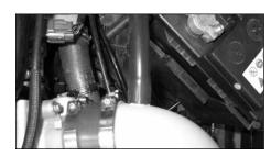
23. Fit the other end of the breather hose onto the vent on the intake tube as shown. If necessary, trim the hose for best fit and clearance.
