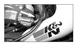
25. Secure the throttle cable to the wiring loom using a cable tie supplied.
