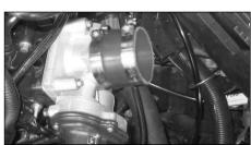
14. Fit the silicone sleeve onto the throttle body using a #44 hose clamp supplied.
