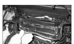
9. Remove the breather assembly from the engine as shown.
