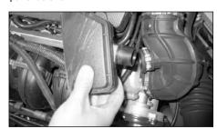
3. Unclip and remove the small resonator box from the air box and intake hose as shown.
