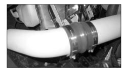
17. Feed the "B" tube into the hump hose using a #44 hose clamp supplied. (Do not fully tighten at this moment.)
