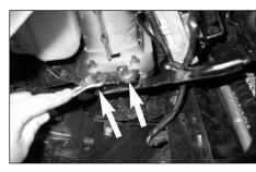
10. As per manufacturer's instructions carefully raise the front of the vehicle and support it with a pair of axle stands. Remove the two indicated nuts that secure the resonator box to the vehicle as shown.
