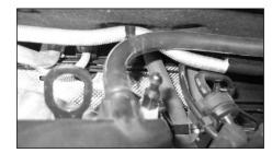
22. Fit the breather hose supplied onto the breather on the cam cover as shown.
