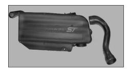
26. Remove the intake tube from the air box as shown.
