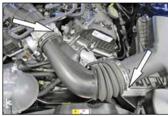
3. Loosen the hose clamps securing the factory intake tube to the throttle body and air filter housing then remove the intake tube from the vehicle.
