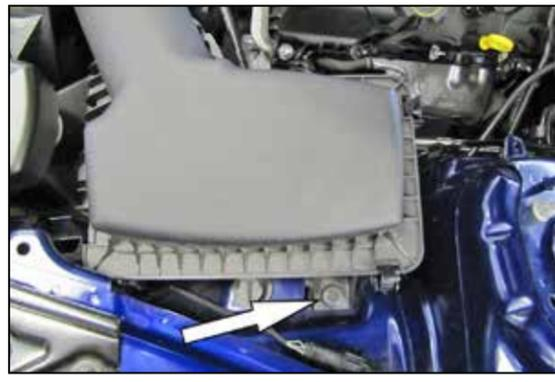
4. Remove the bolt which secures the air filter housing to the inner fender and then remove the air filter housing from the vehicle.
