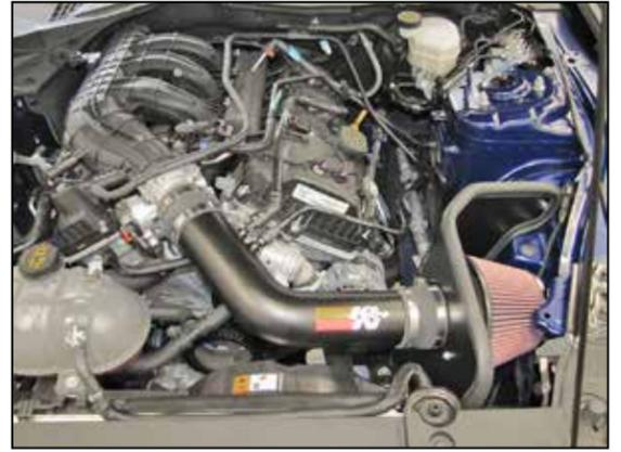
16. Reconnect the vehicle's negative battery cable. Double check to make sure everything is tight and properly positioned before starting the vehicle.
