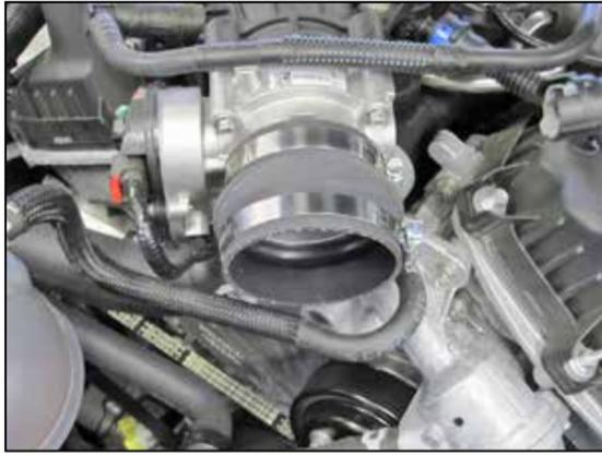
11. Install the provided hump coupler (028171) onto the throttle body and secure with the provided hose clamp.
