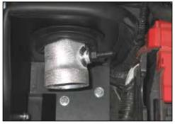
28. When equipped with EVAP, pass the K&N® intake tube through the heat shield and rotate so the remaining  $\frac{1}{2}$ "npt vent fitting can be installed as shown.
