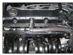
22a. **Non US models:** Install the provided  $\frac{1}{2}$ " silicone vent hose onto the  $\frac{1}{4}$ " vent and guide it along the fuel line towards the intake tube.
