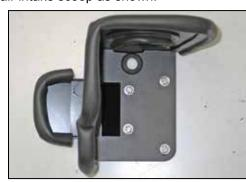
17. Attach the fresh air scoop to the heat shield using the provided hardware.
