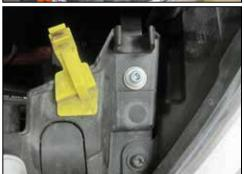
9. Install the provided 30mm long Allen bolt and washer into the air box mounting bracket hole as shown. On some models it may be necessary to use the supplied larger washer.
