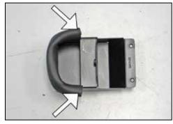
16. Install the 7" section of edge trim onto the fresh air intake scoop as shown.
