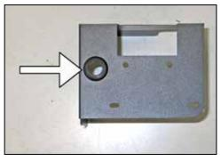
11. Install the provided grommet into the bottom of the heat shield as shown.
