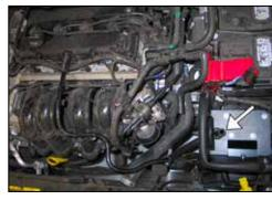
22. **US Models Only:** Reinstall the crankcase vent hose assembly onto the valve cover and route the silicone hose through the grommet in the bottom of the heat shield.
