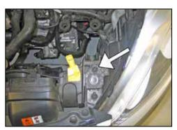
8. Remove the airbox mounting bracket bolt shown.
