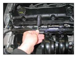
21a. Remove the rubber hose from the crankcase vent assembly and attach it to the valve cover as shown. Install the 1/4" 90° vent into the rubber hose as shown."
