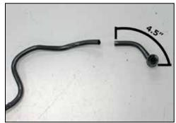
20. **US Models Only:** Measure back 4.5" from the end of the crankcase vent tube then cut the tube as shown.
