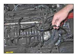
5. Release the locking collar for the crankcase vent hose to the airbox connection by pulling it back, so the crankcase vent hose can be disconnected from the airbox. Then disconnect the crankcase vent hose from the valve cover and remove it from the vehicle.
