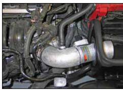
30. When equipped with EVAP, install the EVAP vent hose to the npt vent fitting.
