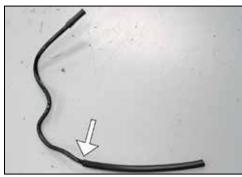
21. **US Models Only:** Install the provided ½" silicone vent hose onto the cut vent tube as shown.
