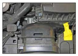
6. Disconnect the fresh air intake scoop from the core support.
