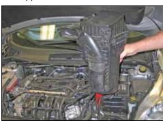
7. Lift up the airbox assembly to dislodge it from the mounting grommets and then remove it from the vehicle.
