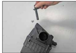
25. Remove the two bolts securing the mass air sensor to the factory airbox and then remove the mass air sensor from the airbox.
