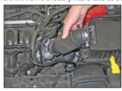
4. Loosen the two hose clamps that secure the factory intake tube and then remove the intake tube from the vehicle.
