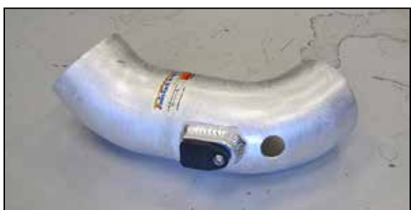
17A. On vehicles equipped with the round style sensor, mark the intake tube as shown 1.0 to 1.25" from the sensor boss. Drill a 3/4" id hole on the mark.
