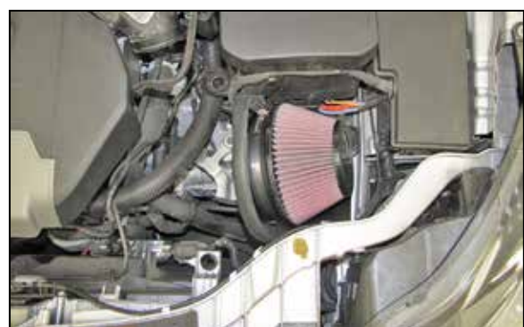
12. Install the K&N® air filter onto the filter adapter and secure with the provided hose clamp.
