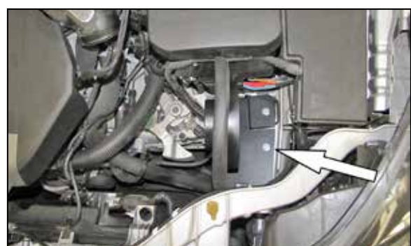
11. Install the heat shield assembly into the engine compartment and secure it to the rubber mounted stud with the provided hardware.
