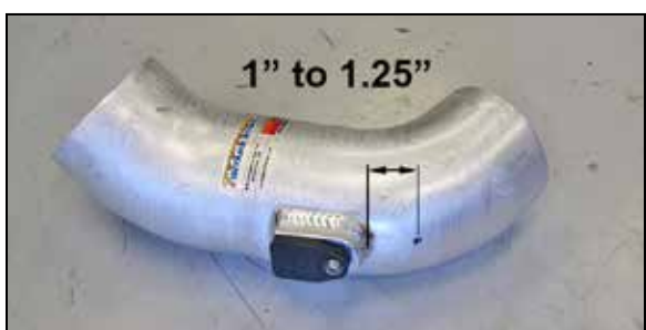
17. Install the pressure sensor into the K&N® intake tube and secure with the provided hardware. NOTE: On vehicles that are not equipped with the temperature sensor secured with the bolt, install the provided block off and O-ring seal.
