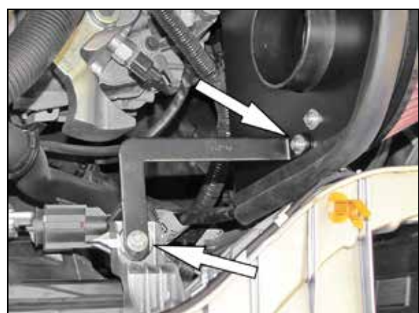
13. Install the heat shield mounting bracket (064311) onto the heat shield and core support with the provided hardware.
