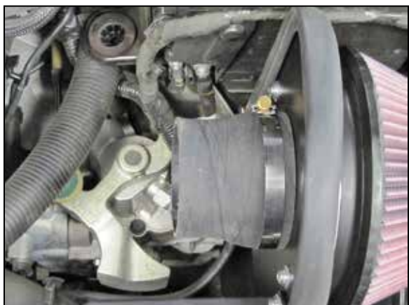
15. Install the provided coupling hose #084055 onto the filter adapter as shown and secure with the provided hose clamp.
