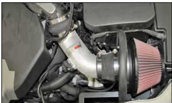
18. Install the K&N® intake tube into the hose at the plenum and then into the hose at the filter adapter and then secure with the provided hose clamps.
