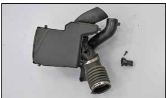
16. Remove the pressure sensor from the factory air box as shown.
