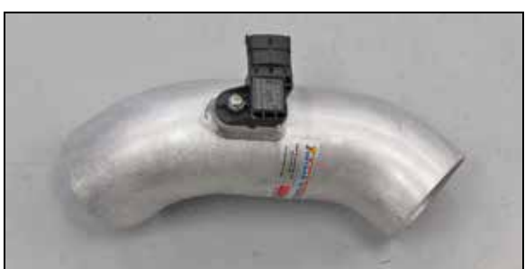
17. Install the pressure sensor into the K&N® intake tube and secure with the provided hardware. NOTE: On vehicles that are not equipped with the temperature sensor secured with the bolt, install the provided block off and O-ring seal.
