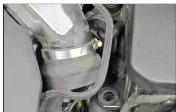
14. Install the coupling hose #08696 onto the plenum and secure with the hose clamp.
