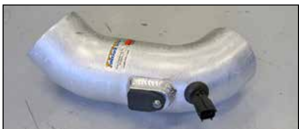
17b. Install the provided grommet into the hole drilled. Then remove the O-ring from the sensor and install the sensor into the grommet. NOTE: The sensor is very fragile, use care while handling the sensor.
