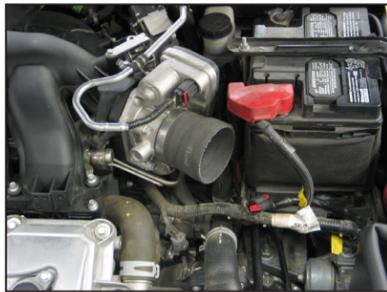
18. Install the silicone hose (08713) onto the throttle body and secure with the provided hose clamp.
