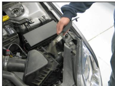
6. Remove the rubber air flap from behind the head light assembly as shown.
