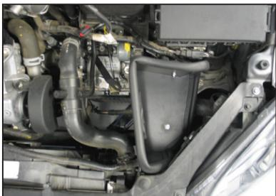
17. Set the heat shield into position on the frame rail and secure with the provide hardware. Secure the rear of the heat shield to the mounting bracket with provided hardware.
