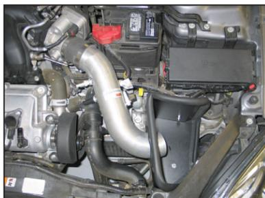
20. Install the K&N® intake tube into the silicone hose at the throttle body and align with the mounting bracket installed in step #12. Secure the intake tube with the hose clamp and hardware provided.
