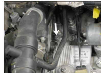
11. Remove the ground strap mounting bolt shown from the transmission.
