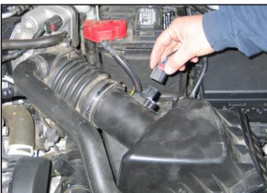
2. Disconnect mass air sensor electrical connection.
