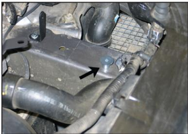
16. Place the heat shield spacer and fender washer onto the frame rail at the front air box mounting location as shown.
