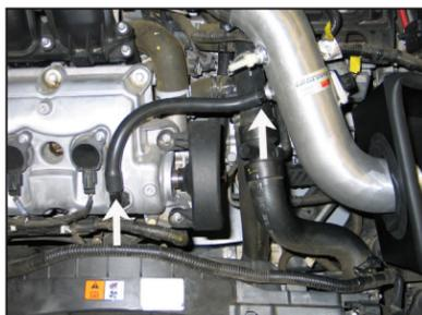
21. Install the provided crank case vent hose onto the valve cover port and then onto the 1/4" NPT fitting installed into intake tube as shown.
