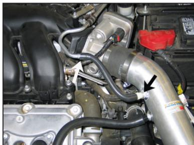
22. On vehicles equipped with an EVAP vent line, install the provided EVAP hose onto the port and then onto the 1/4" NPT fitting installed into the K&N® intake tube as shown.
