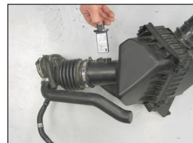
9. Remove the two screws that retain the mass air sensor and then remove the mass air sensor from the air box.
