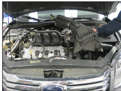
7. Lift up the air box to dislodge it from the mounting grommet and then remove the complete intake assembly.
