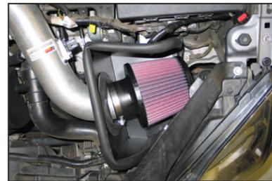
23. Install the K&N® air filter and secure with the provided hose clamp.
