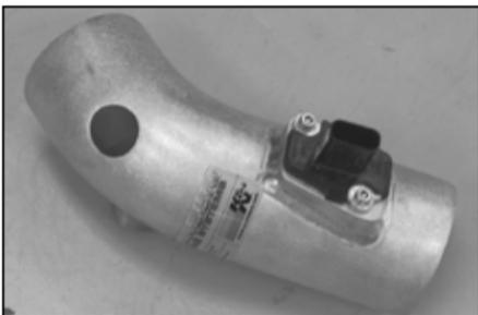
21. Install the mass air sensor into the K&N® intake tube, then fasten using the provided hardware.
