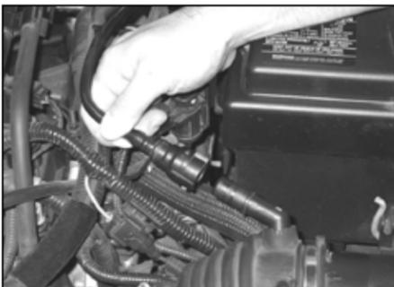
2. Remove the crankcase vent hose by pressing the green locking tab and gently pulling the crankcase vent hose away from the fitting.
