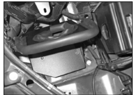
18. Place the heat shield into position onto the inner fender well heat shield mounting bracket and align the second heat shield bracket with the threaded hole in the inner fender. Fasten the heat shield using the provided hardware.
