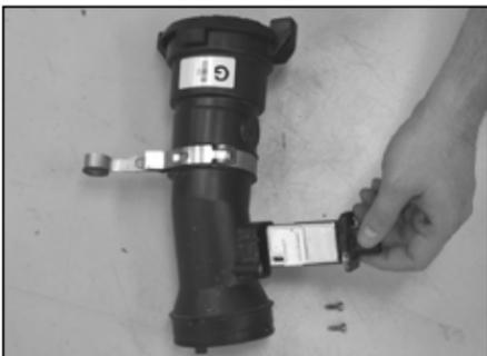
20. Remove the two screws that fasten the mass air sensor to the mass air sensor housing, then remove the mass air sensor from the housing.
