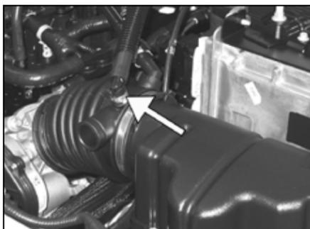
3a. On vehicles equipped with an EVAP vent line, cut the clamp that secures the vent line elbow to the stock intake tube. Then, remove the EVAP vent from the intake tube as shown.
