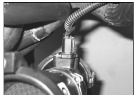
6. Disconnect the mass air sensor electrical connection. Press the locking tab, then gently pull away from the housing.
