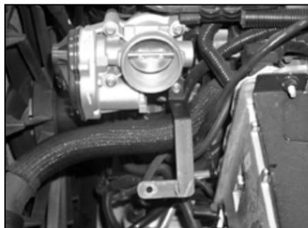
13a. On 2009 models, install the tube mounting bracket (083133) onto the throttle body and secure with the factory mounting bolt from step 12a.
