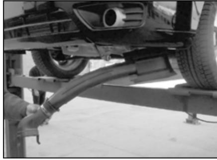
11. On vehicles equipped with the upper intake snorkel, pull down on the snorkel to dislodge it from the mount and then remove it from behind the fender.
