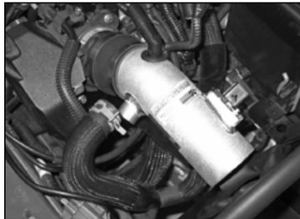
24. Install the K&N® intake tube into the silicone hose previously installed onto the throttle body. Align the intake tube with the previously installed intake tube mounting bracket; fasten using the respective hose clamp and hardware.
