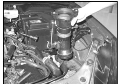
8. Loosen the hose clamp that fastens the mass air sensor housing to the air filter housing, then remove the mass air sensor housing.
