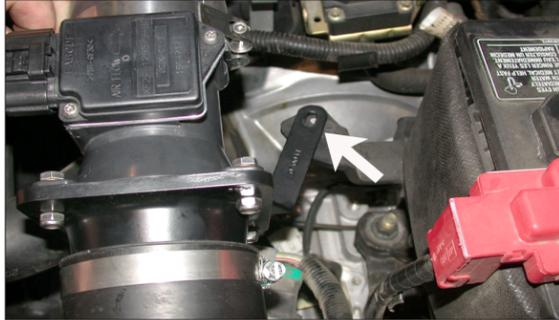
19. Slide the mass air sensor assembly into the silicone step hose, then, line up the bracket with the hole located on the battery tray as shown.
