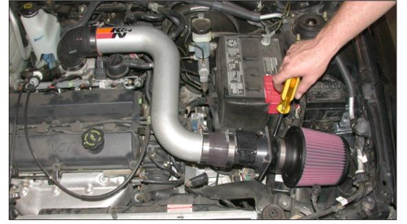
22. Install the air filter and secure with the provided hose clamp as shown.
