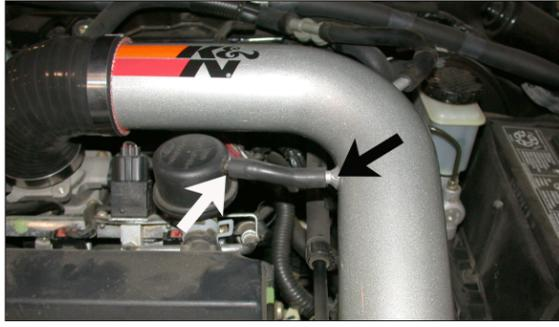
16. Connect the provided hose onto the cam cover vent and to the vent on the intake tube as shown.
