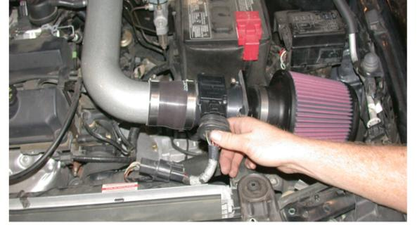
23. Reconnect the secondary and primary mass air electrical connections as shown.
