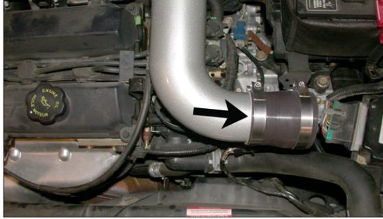
17. Install the silicone step hose and hose clamps onto the intake tube as shown.
