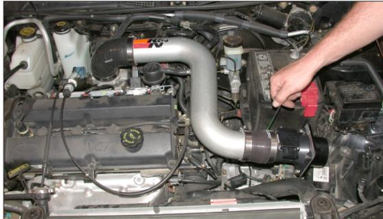
21. Tighten all hose clamps and hardware and adjust for best fit.
