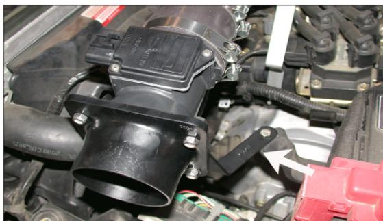
20. Secure the bracket to the battery tray using the provided hardware as shown.
