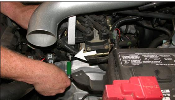
15. Secure the bracket to the stud using the provided washer and hex nut as shown.
