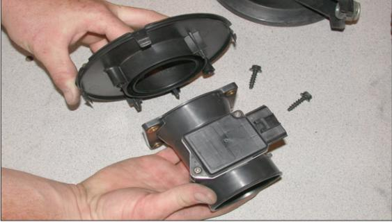
11. Remove the two bolts that secure the mass air sensor, then, remove the mass air sensor as shown.
