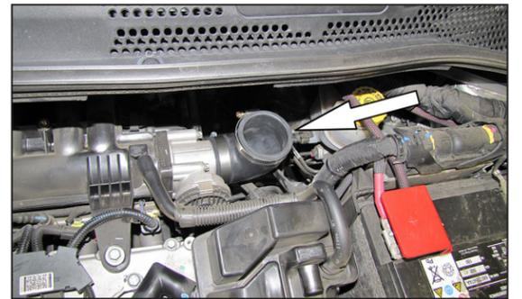
8. Install the provided elbow hose (03108) onto the throttle body as shown.
