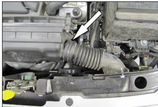
5. Disconnect the fresh air intake hose from the intake plenum.
