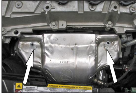
15. Install the two nut extensions onto the heat shield mounting studs as show.
