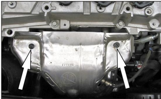
14. Remove the two exhaust manifold heat shield nuts shown.
