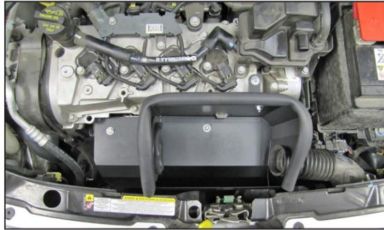
16. Set the heat shield onto the nut extensions, snap the fresh air duct into the heat shield and then secure the heat shield to the nut extensions and valve cover with the provided hardware.
