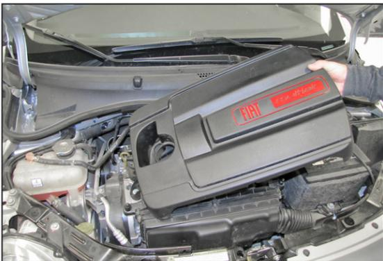
2. Lift up the engine cover and remove it from the engine.
