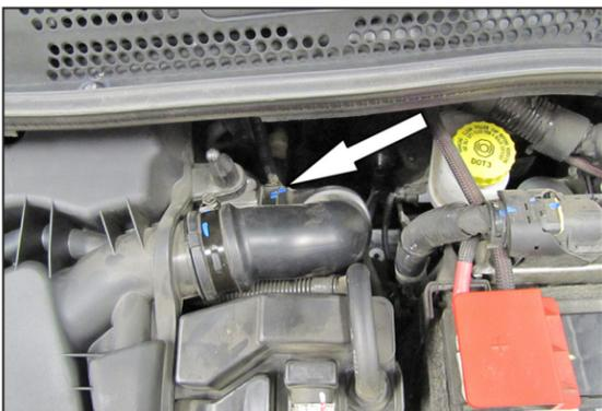
3. Loosen the hose clamp securing the intake tube to the throttle body.
