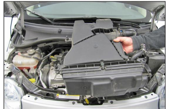
7. Lift up and remove the complete stock intake system from the engine.
