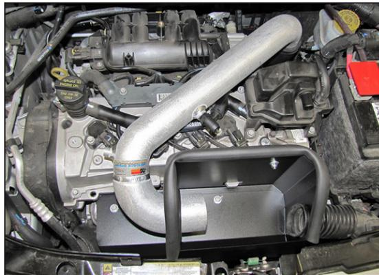
18. Install the K&N® intake tube into the heat shield and then into the silicone hose at the throttle body.
