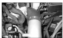
16. Slide the A -tube into the silicone hose using a #44 hose clamp supplied. Do not fully tighten yet!
