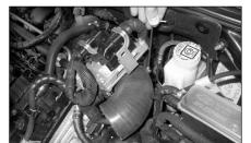
15. Mount the 90 degree silicone hose onto the throttle body using a #44 hose clamp supplied. Do not fully tighten yet!
