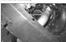
26. Align the tubes and filter for best fit and clearance, then, firmly tighten all hose clamps and hardware connections.
