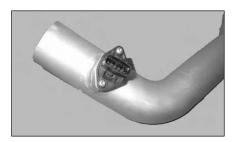
14. Install the MAS into the A-tube using the two M5 screws supplied.
