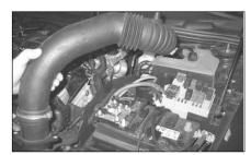
5. Unscrew and remove the complete intake tube including the MAS from the throttle body as shown
