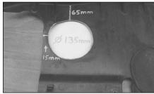
22. Cut a hole into the left under tray (removed in step 8) with a diameter of approx. 135mm at 65mm from the top and 15mm from the side as shown
