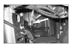
12. Screw the rubber vibration stud into the air box mounting point underneath the battery tray as shown
