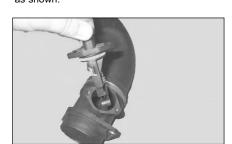
6. Unscrew and carefully remove the MAS from the intake tube as shown
