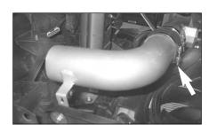
20. Fit the B-tube into the silicone hump hose using a #44 hose clamp supplied. Do not fully tighten yet!
