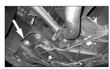
13. Remove the left rubber grommet and mount the rubber stud using the two large washers and the M6 nylock nut supplied. Make sure to fit a large washer either side of the hole & do not fully tighten yet!
