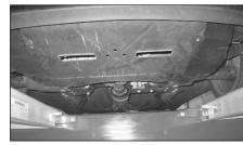
27.Re-install the center under tray to the vehicle using its original hardware.
