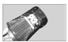
24. Fit the Drycharger around the filter. **NOTE:** The Drycharger's water repellant properties will last up to two years. See the parts list to re-order Drycharger if necessary.
