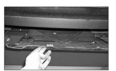
7. Taking the necessary safety precautions as per manufacturer's instruction raise the front of the vehicle . Remove the center under tray from the vehicle as shown.
