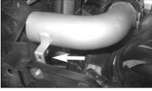
21. Align the bracket of the B-tube with the rubber stud and secure using an M6 washer and M6 nylock nut supplied. Do not fully tighten yet!
