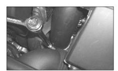
4. Unscrew the bolts that attach the Mass Air Sensor (MAS) to the airbox, and unclip the electrical harness from the MAS.
