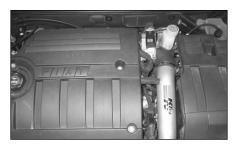
29. Reconnect the negative battery terminal, re-install the battery cover and the engine cover using their original hardware. Installation is now complete.
