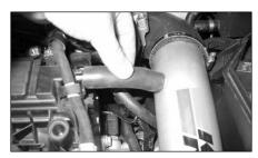
28. Fit the silicone breather hose provided between the engine's vent and the vent on the A-tube as shown.
