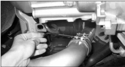
25. Align the B-tube assembly for best fit and clearance, then, tighten the #275 barrel clamp and nut securing the weld-on bracket.
