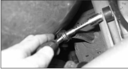
24. Fit the weld-on bracket on the B-tube onto the rubber mounting stud using the flat metal washer and nylock nut supplied as shown. Don't fully tighten yet!
