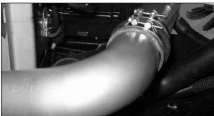
23. Fit the B-tube assembly into the silicone hump hose using the #275 barrel clamp supplied. Do not yet fully tighten the barrel clamp.
