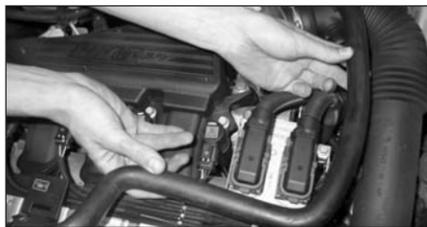
3. Unclip and remove the breather hose from engine and intake hose as shown.
