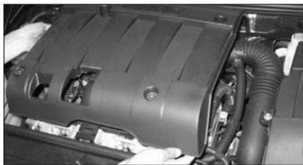
2. Undo the 4 bolts & remove the engine cover.
