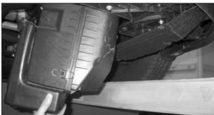
9. Unbolt the air box mounting bolt (underneath the battery tray) and carefully remove the air box from the vehicle leaving the intake snorkel in place.
