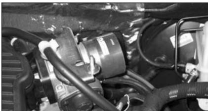
10. Fit the silicone hose to the throttle body using the #250 barrel clamp supplied. To tighten, use the Allen Head wrench supplied.
