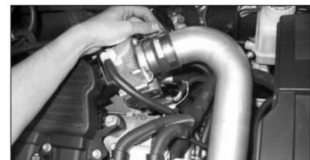
13. Fit the K&N Typhoon intake A-tube into the silicone hose, using the #275 barrel clamp. Do not yet tighten the #275 barrel clamp.
