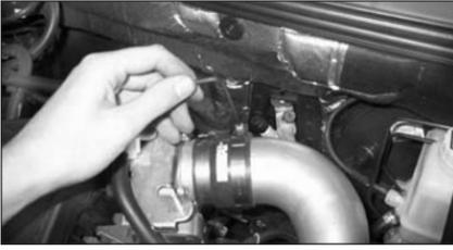
15. Tighten the #275 barrel clamp.
