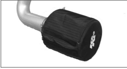
21. Fit the Drycharger over the filter element as shown. **NOTE:** The Drycharger's water repellent properties will last up to 2 years. See parts list to re-order Drycharger if necessary.
