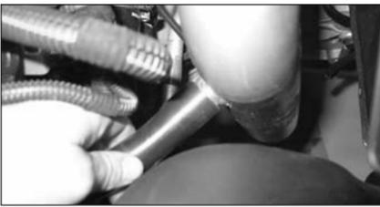
17. Fit the other end of the silicone breather hose onto the breather pipe on the A-tube. For easier fitment, you may want to slightly grease the silicone hose and the pipe.
