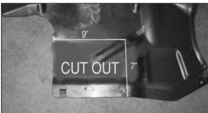
26. With a box cutter, cut out a piece of the left mud guard (removed in step 7) of 9 by 7 inches (229 by 178 mm) as shown.
