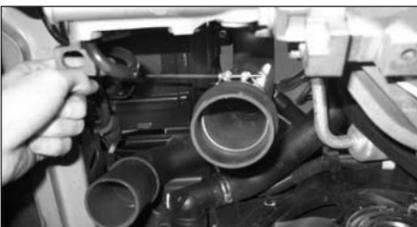
19. From the underside of the car, fit the silicone hump hose to the intake tube using the #275 barrel clamp supplied.
