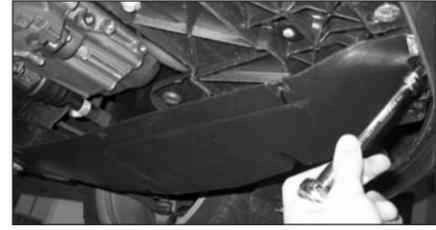
27. Re-install the left mud guard and the under tray to the car.
