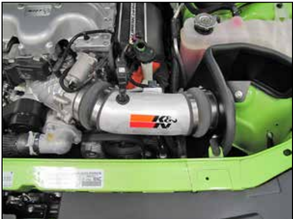
16. Install the K&N® intake tube assembly into position, Slide the coupling hoses out and onto the throttle body and filter adapter. Then adjust the tube and hoses for proper fit and secure with the provided hose clamps.
