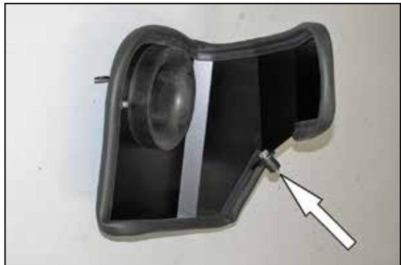
10. Install the Inserted nut onto the heat shield as shown.
