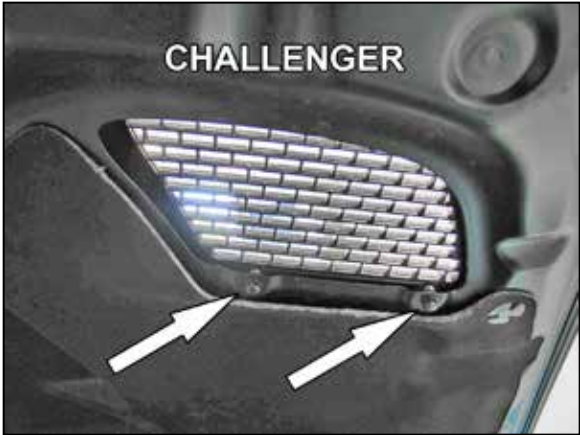
19. Install the K&N® air filter and secure with the provided hose clamp. NOTE: Drycharger® air filter wrap; #RF-1041DK is available separately and is recommended if the vehicle is to be used in inclement weather. Protection of the air filter is recommended while washing the vehicle as the filter is exposed under the hood grill.
