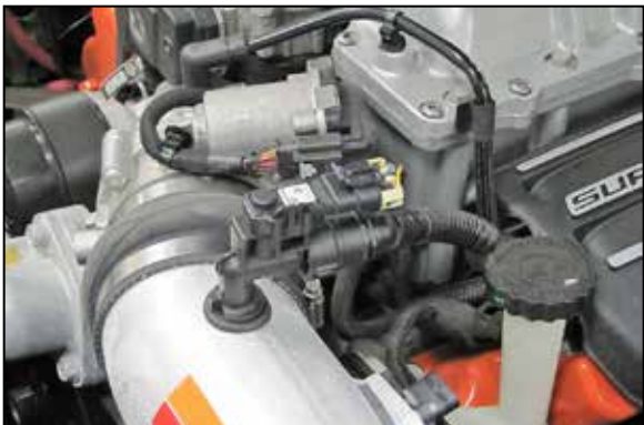
17. Reconnect the crank case vent hose and pressure sensor electrical connection. NOTE: Rotate the K&N® intake tube towards the rear of the vehicle and slide it towards the throttle body to provide the maximum amount of hood clearance, additional clearance can be achieved by rotating the crank case vent hose to adjust its position.
