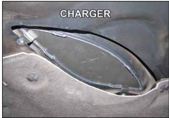
21. Install the shield under the factory vent grid so the mounting tabs are between the hood and the grid as shown.
