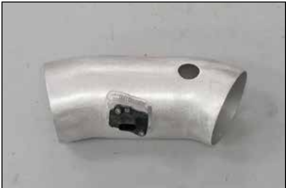
13. Install the mass air sensor into the K&N® intake tube and secure with the provided hardware.
