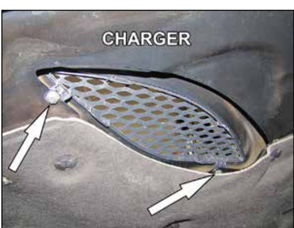
20. If the vehicle is to be driven during inclement or wet weather it is recommended the shield be installed onto the hood vent to guard the air filter from concentrated water. Remove the two bolts that secure the factory vent grid.
