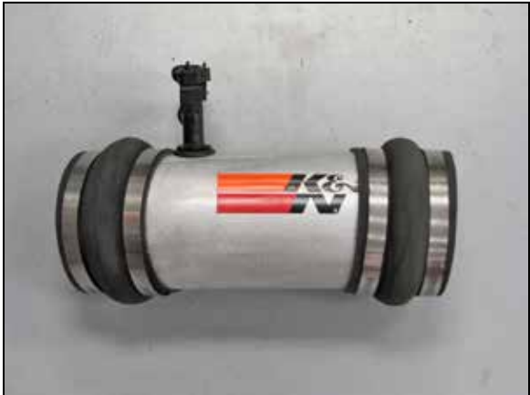
15. Install both of the coupling hoses (08418) onto the K&N® intake tube as shown. NOTE: Install the hose as far onto the tube as possible to aid the installation onto the vehicle.
