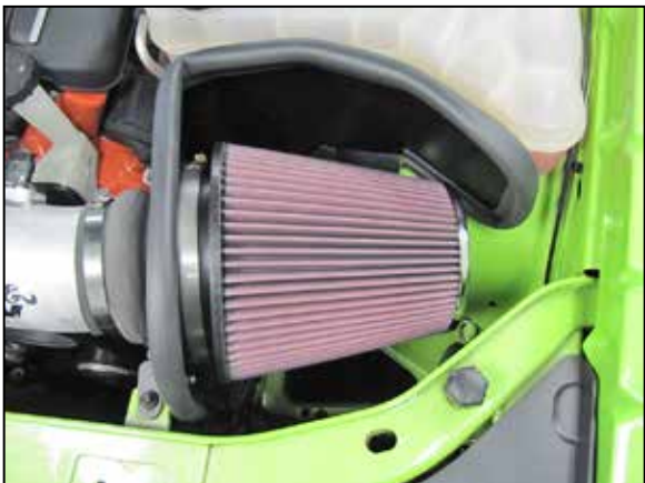
19. Install the K&N® air filter and secure with the provided hose clamp. NOTE: Drycharger® air filter wrap; #RF-1041DK is available separately and is recommended if the vehicle is to be used in inclement weather. Protection of the air filter is recommended while washing the vehicle as the filter is exposed under the hood grill.
