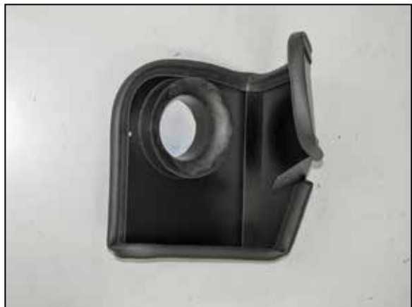
8. Install the provided edge trim onto the heat shield as shown. NOTE: Trimming of the edge trim will be necessary.
