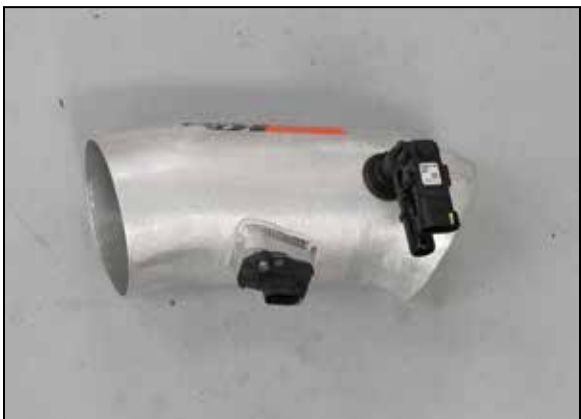
14. Install the provided grommet and pressure sensor/sensor/vent assembly into the K&N® intake tube as shown.
