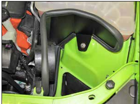
11. Install the heat shield assembly into the vehicle so the insert nut goes into the factory air box grommet mount. Secure the bracket to the core support with the factory bolt from step #6 and tighten the bolt into the insert nut.
