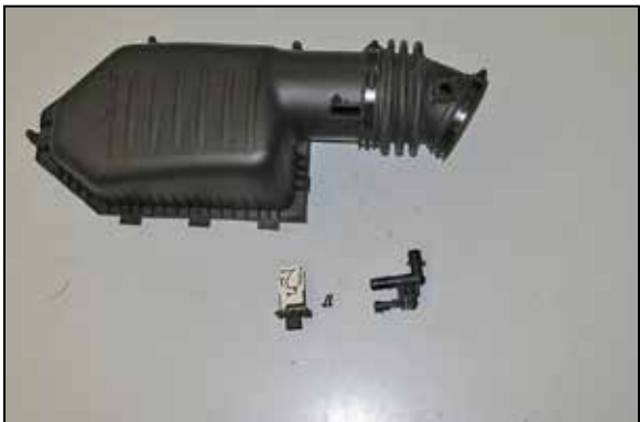
12. Remove the two screws securing the mass air sensor into the air filter housing and then remove the mass air sensor. Remove the pressure sensor/vent assembly from the factory intake hose as shown.
