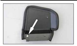
12. Install one of the provided brackets #070812 onto the heat shield as shown using the provided hardware.
