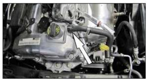
8. Remove the crank case vent hose from the valve cover port
