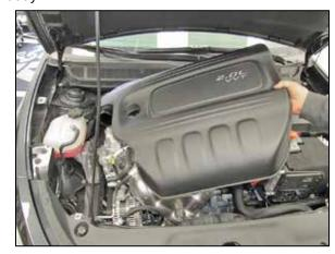
7. Lift up and remove the intake plenum from the vehicle.
