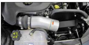
21. Install the K&N® intake tube into the silicone hose and align with the mounting bracket previously installed. Secure the tube with the provided hardware and hose clamp.
