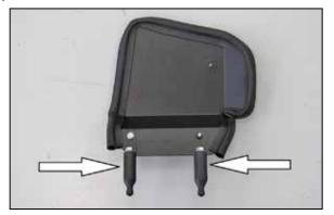
14. Install the two heat shield mounts onto the brackets as shown.
