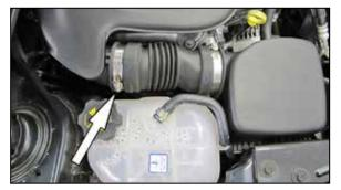
2. Loosen the hose clamp securing the intake hose to the intake plenum.
