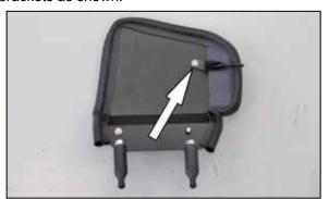
15. Install the final heat shield mounting bracket #07139 onto the heat shield and secure using the provided hardware.
