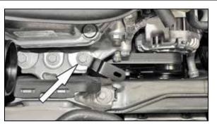
17. Install the tube mounting bracket #064301 onto the engine mount and secure with the factory bolt from the previous step.
