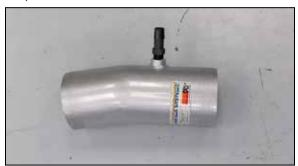
20. Install the crank case vent fitting into the K&N® intake tube as shown.
