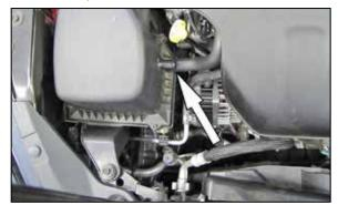
3. Disconnect the crank case vent hose from the air filter housing
