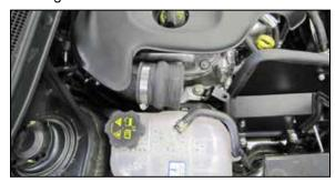
19. Install the provided hump hose #08696 onto the plenum inlet and secure with the provided hose clamp.
