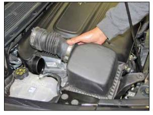
5. Lift up and remove the air filter housing assembly from the vehicle.
