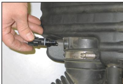
17. Remove the inlet air temperature sensor from the stock intake tube.
