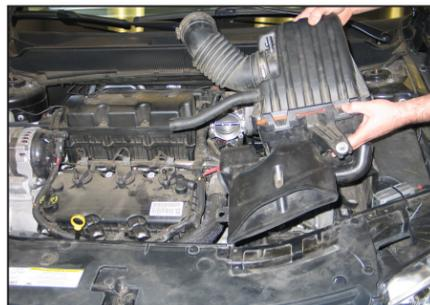
7. Loosen the intake tube hose clamp and disconnect the intake tube from the throttle body. Then lift up and remove the complete stock intake assembly.
