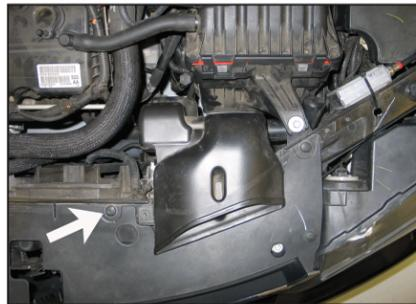
4. Remove the plastic retaining clip which secures the fresh air intake scoop to the core support.
