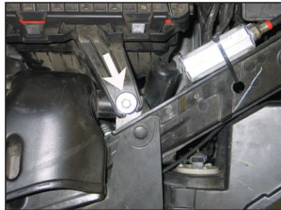
5. Remove the airbox retaining bolt shown. This bolt will be reused in a later step.
