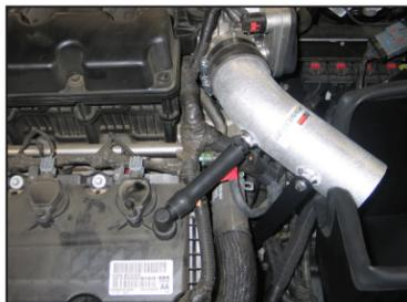
22. Install the provided crankcase vent hose onto the fitting on the valve cover. Then connect the open end to the NPT fitting installed into the K&N® intake tube.
