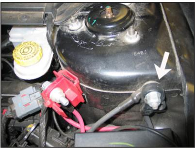
1. Turn off the ignition and disconnect the negative battery cable at the junction on the strut tower.
