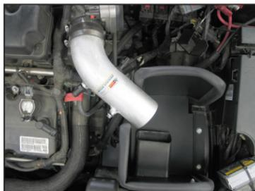
21. Install the K&N® intake tube into the silicone hose at the throttle body, aligning the tube with the mounting bracket. Secure with the provided hose clamp and hardware provided.
