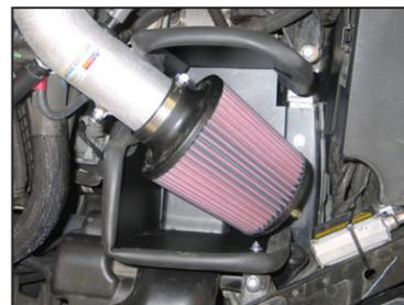
24. Install the K&N® air filter onto the intake tube and secure with the provided hose clamp.
