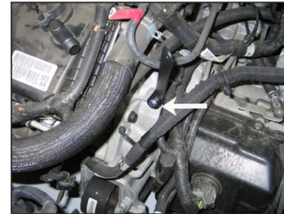
9. Install the tube mounting bracket (070117) onto the transmission case using the provided hardware.
