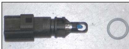
18. Remove the o-ring from the temperature sensor as shown.
