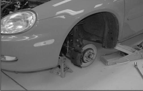
11. Jack the driver's side of the vehicle up and support with jack stands then remove the tire.
