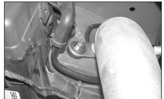
25. Using the supplied nut, tighten the intake tube bracket to the stock stud.
