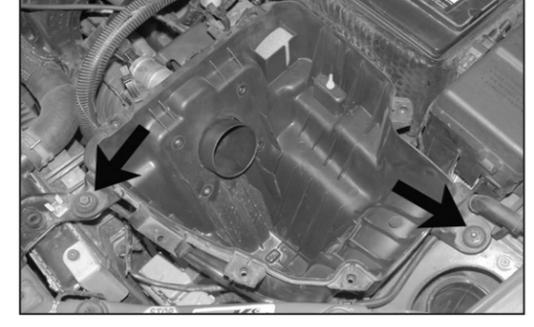
9. Remove the bolt and nut that secure the the air box to the vehicle. Bolt will be re-used.
