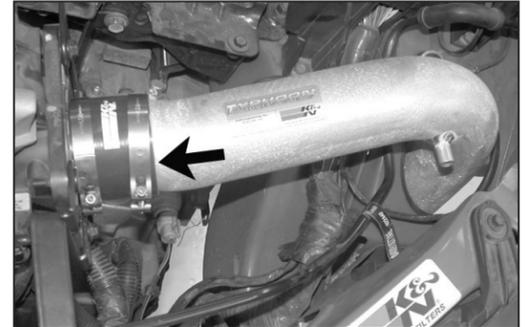
23. Slide the intake tube down the resonator hole then insert the other end into the throttle body silicone hose.
