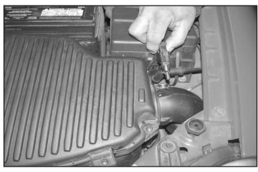
2. Remove the air temperature sensor from the stock intake tube as shown
