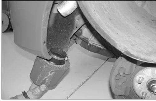
30. From underneath the vehicle, install the K&N® air filter onto the intake tube.
