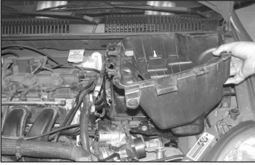
10. Remove the air box from the vehicle.
