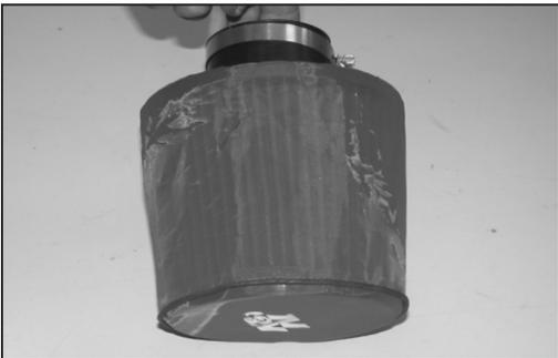
29. Install the K&N® Drycharger® and hose clamp onto the K&N® air filter.
