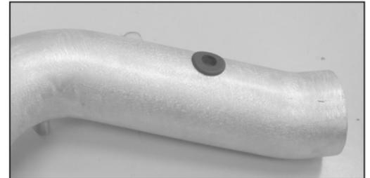
22. Install the smaller grommet into the intake tube.
