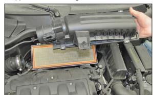
6. Remove the upper air filter housing and air filter. NOTE: K&N Engineering, Inc., recommends that customers do not discard factory air intake.
