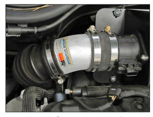
13. Install the K&N® intake tube into the factory hose and then into the hose at the throttle body, then secure with the factory and provided hose clamps.
