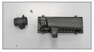
7. Remove the two bolts that secure the mass air sensor to the upper housing and then remove the mass air sensor.
