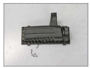
10. Remove the four upper housing mounting
