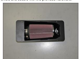
9. Install the K&N $^{\!0}$  air filter onto the mass air sensor and secure with the provided hose clamp.
