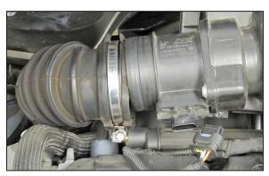
4. Disconnect the intake hose from the mass air sensor.
