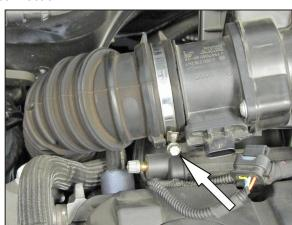
3. Loosen the hose clamp that secures the intake hose to the mass air sensor.
