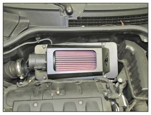
11. Install the K&N® filter assembly onto the lower air filter housing and secure with the factory screws from step #10.
