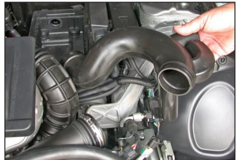
8. Remove the air cleaner inlet duct as shown.
