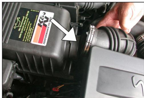
3. Pull the stock intake tube off the air cleaner as shown.
