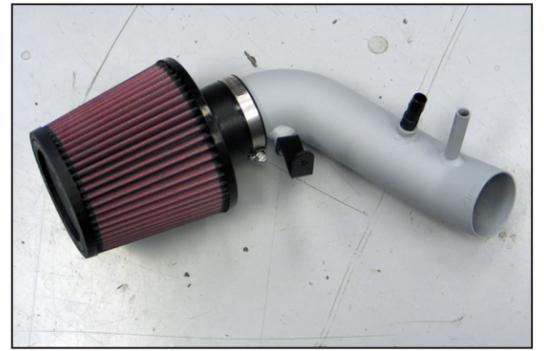
21. Install the K&N® air filter onto the K&N® intake tube and tighten with the provided hose clamp as shown.
