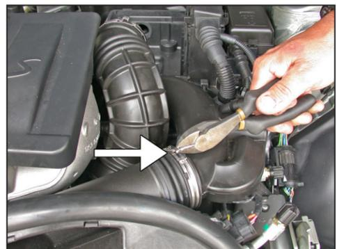
7. Using a pair of dikes or pliers unclip the hose clamp on the air inlet duct as shown.
