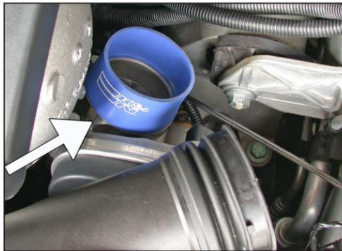
19. Install the silicone hose and the provided hose clamp onto the throttle body and tighten as shown.
