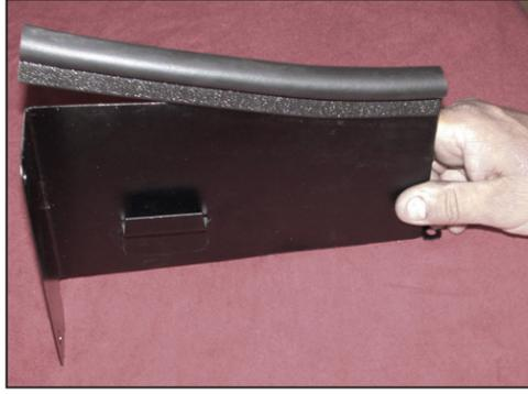
15. Install the provided edge trim onto the K&N® heat shield as shown.
