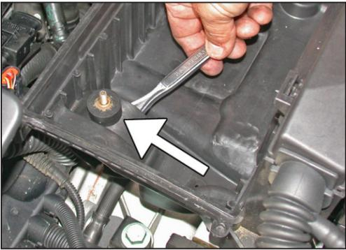
13. Secure the provided rubber mounted stud to the air inlet flange on the lower air cleaner assembly using the provided hardware as shown.
