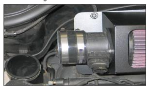
15. Install the provided silicone hose (08756) onto the mass air sensor and secure with the provided hose clamp.
