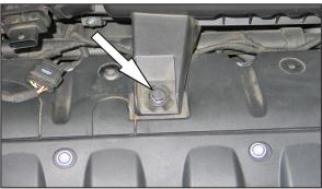
5. Loosen the bolt which secures the upper air box to the valve cover.
