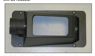
11. Using the provided hardware, secure the factory mass air sensor to the K&N® heat shield as shown.
