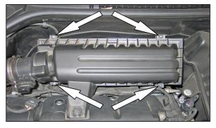
4. Loosen the four screws which secure the upper air box housing to the lower air box housing.
