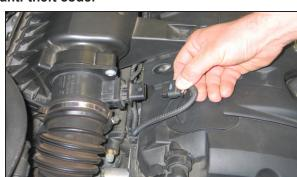
2. Release the locking tab and then disconnect the mass air sensor electrical connection.
