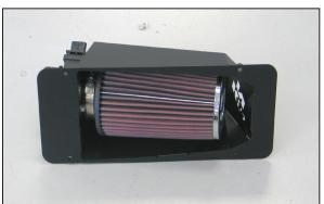
12. Install the K&N<sup>®</sup> air filter onto the mass air sensor and secure with the provided hose clamp.
