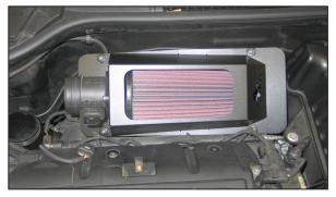
14. Install the heat shield/filter assembly onto the lower air box and secure with the four factory upper air box retaining screws.
