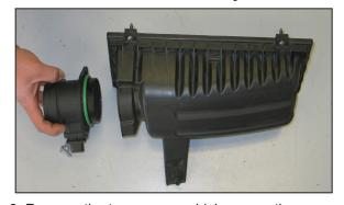
8. Remove the two screws which secure the mass air sensor to the upper air box and then remove the mass air sensor.
