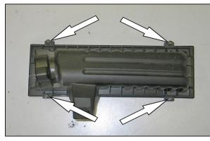
10. Remove the four upper air box retaining screws from the upper air box.
