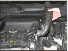
5. Remove the stock intake tube from the vehicle. NOTE: K&N Engineering, Inc., recommends that customers do not discard factory air intake.
