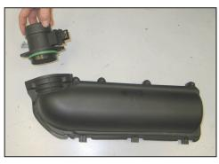
7. Remove the two screws which secure the mass air sensor to the upper airbox and then remove the mass air sensor from the upper airbox.
