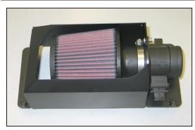
10. Install the K&N® air filter onto the mass air sensor inside the heat shield and secure with the provided hose clamp.
