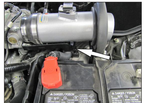
21. Using the provided tie wrap, Secure the wiring harness to the tube mounting bracket.
