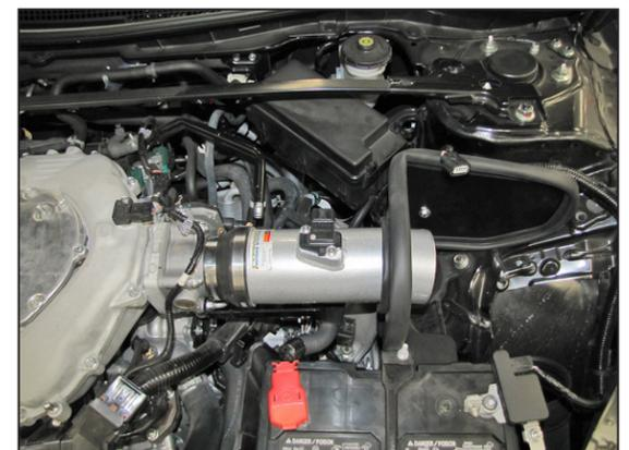
20. Install the K&N® intake tube through the heat shield and then into the silicone hose, and then align with the mounting bracket. Secure the tube with the provided hose clamp and hardware.
