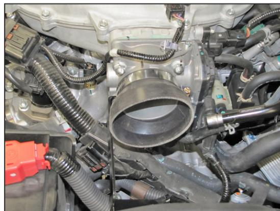
16. Install the appropriate step hose onto the throttle body and secure with the provided hose clamp.
