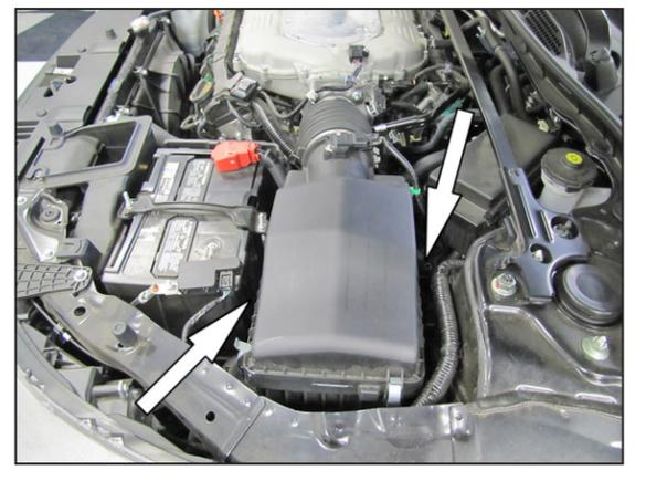
6. Loosen and remove the two air box mounting bolts.
