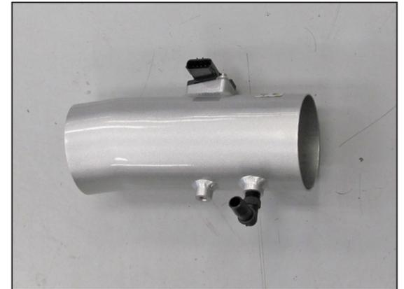
19. Install the 90° vent fitting into the K&N® intake tube as shown.
