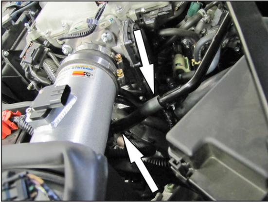
22. Connect the provided crank case vent hose to the factory vent tube and then connect the open end to the 90° vent fitting installed into the K&N® intake tube.
