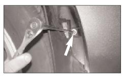
24. From the side of the vehicle loosen and remove the second bolt on the resonator as shown.
