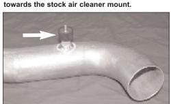
28. Install the provided rubber mounted stud onto the threaded boss on the K&N® intake tube.
