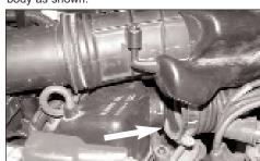
6. Loosen the hose clamp on the resonator then disconnect the flange as shown. (VTEC only)
