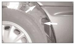
20. Remove the two push clips on the inner wheelhouse valance as shown.
