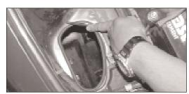
35. Apply the edge trim on the inner fender as shown. Trim if necessary.
