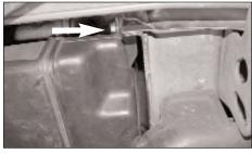
23. From below the vehicle, loosen and remove the first bolt on the air cleaner resonator as shown.
