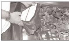
Pull upwards to remove the lower air cleaner assembly as shown.
