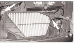
8. Remove the two bolts that secure the lower air cleaner assembly as shown.
