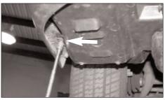
19. Raise the vehicle and support it with jack stands then remove the bolt on the lower valance as shown.
