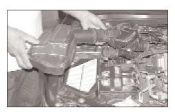
7. Remove the four bolts on the upper air cleaner assembly, then, pull upwards to remove the upper air cleaner assembly and stock intake tube as shown.
