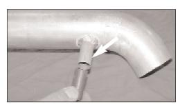
29. Install the provided silicone hose into the vent on the K&N $^{\tiny \circledR}$  intake tube as shown.
