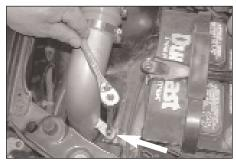
40. Secure the cold air tube bracket to the rubber mounted stud using the provided hardware as shown.
