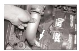
38. Slide the K&N® cold air intake tube into the hole in the inner fender and line up the tube bracket with the rubber mounted stud from step 36.
