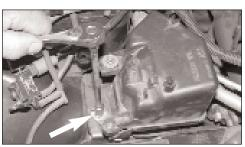
13. Remove the two bolts that secure the resonator
