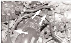
4. Unclip the EVAP vent, throttle cable and the MAP sensor electrical connection from the stock intake tube as shown.
