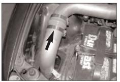
39. Slide the silicone hump hose onto the K&N  $^{\! @}$  cold air intake tube as shown.
