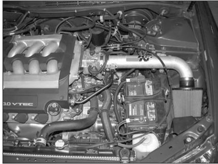
32. This K&N® Typhoon® intake kit has been designed to be used in two different configurations. In the case of inclement weather, the cold air tube can be removed and the filter can be clamped onto the intake tube located in the engine compartment to avoid the possibility of ingesting water into the engine.
