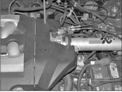
30. Re-install the plastic throttle body cover as shown.
