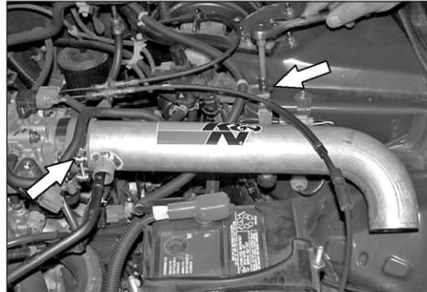
20. Slide the K&N® intake tube into the silicone hose on the throttle body, then, using the bolt removed in step 16, secure the "Z" bracket and the EVAP canister purge valve bracket to the stock mounting point as shown.
