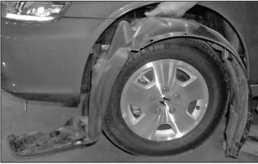
13. Using a flat blade screwdriver and a phillips screwdriver, remove the push clips and screws that retain the inner fender valance, then remove the valance as shown.
