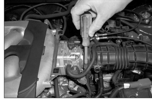
7. Using a phillips screwdriver, loosen the hose clamp at the throttle body as shown.
