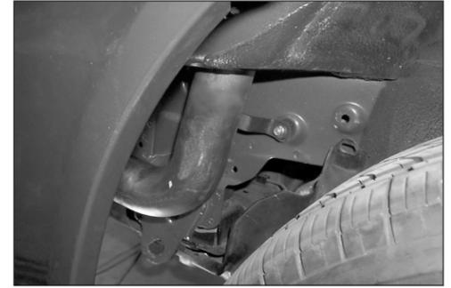
24. Secure the bracket on the K&N® cold air tube to the rubber mounted stud using the provided hardware as shown.
