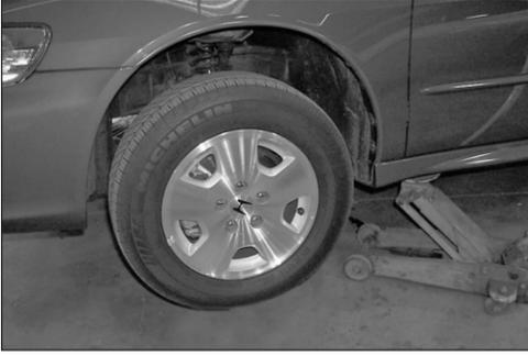
12. Using a floor jack, raise the driver front side of the vehicle up and support the vehicle with jack stands.
