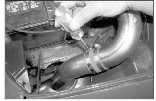
23. Line up the bracket on the cold air tube with the rubber mounted stud in the inner fender, then, secure the K&N® cold air tube to the silicone hump hose.
