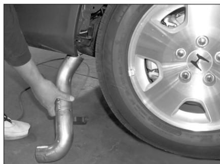
22. Install the K&N® cold air tube from underneath the vehicle as shown.
