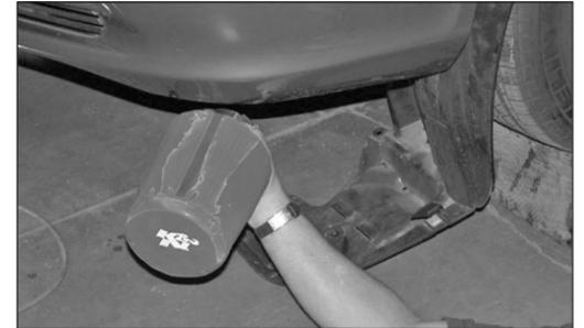
26. Install the K&N® air filter from underneath the vehicle and secure it with the provided hose clamp.
