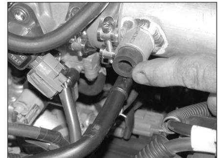
27. Slide the provided rubber sleeve into the vent on the K&N® intake tube.
