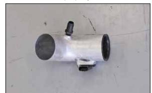
23. Install the provided vent fitting into the K&N® tube as shown.
