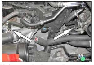
8. Release the spring clamps securing the coolant by-pass hose connections to the engine and then disconnect the coolant by-pass hose and remove the by-pass hose/crank case vent pipe assembly.
