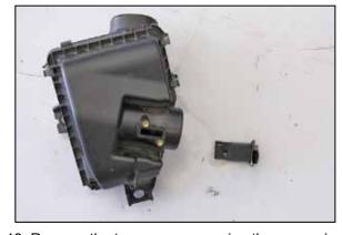
19. Remove the two screws securing the mass air sensor and then remove the mass air sensor from the factory air box.
