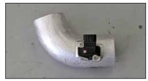
20. Install the mass air sensor into the K&N® intake tube and secure with the provided hardware.
