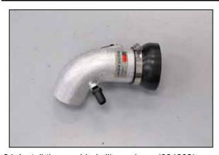
24. Install the provided silicone hose (084093) onto the Intake tube as shown and secure with the provided hose clamp.
