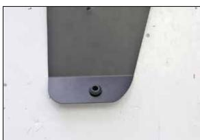
16. Install the mounting grommet into the heat shield as shown.
