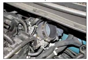
11. Install the provided silicone hose (084016) onto the throttle body and secure with the provided hose clamp.
