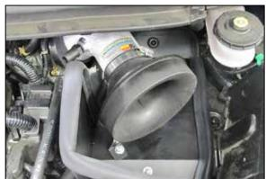
27. Install the filter adapter into the silicone hose on the intake tube and align the bracket with the mounting holes in the heat shield. Secure the bracket with the provided hardware and secure the tube with the hose clamps.
