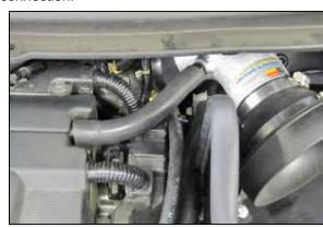
29. Install the provided crank case vent hose onto the vent port of the valve cover and to the fitting installed into the K&N® intake tube.
