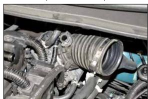
10. Loosen the hose clamp securing the intake hose to the throttle body and remove the intake hose from the throttle body.
