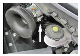
28. Reconnect the mass air sensor electrical connection.
