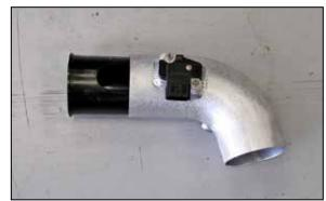
22. Install the mass air senor insert into the K&N® intake tube as shown.
