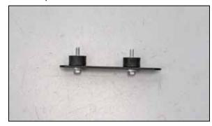
13. Install the two rubber mounted studs onto the provided bracket (083173) as shown and secure with the provided hardware.
