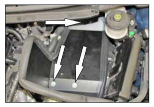
18. Install the heat shield assembly onto the air box mounting stud and rubber mounted studs and then secure with the provided hardware. Secure the fresh air inlet hose to the heat shield with the provided hardware.
