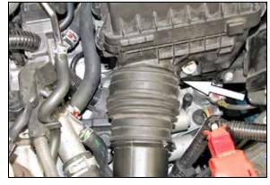
3. Disconnect and remove the fresh air hose from the air box and fresh air inlet, then remove the hose from the vehicle.
