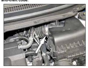
2. Loosen the hose clamp securing the intake tube to the air box and then disconnect the tube from the air box.
