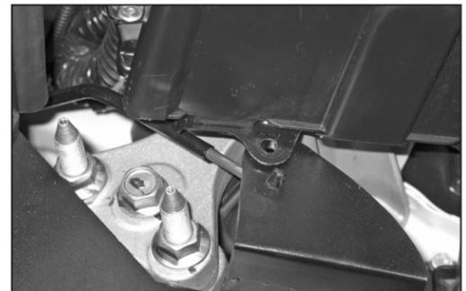
24. Install clip to the hydraulic line then attach to hole in heat shield.
