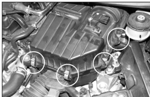
4. Unclip the four clips that secure the upper airbox in place, then remove the upper factory airbox.
