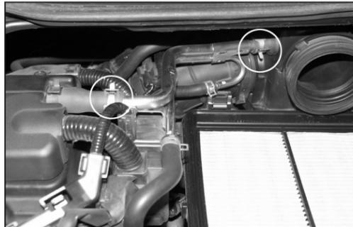
5. Unclip the two clips that secure the CCV-hose (one is located on the engine's valve cover, the other is located on the lower factory airbox) and disconnect the CCV-hose
