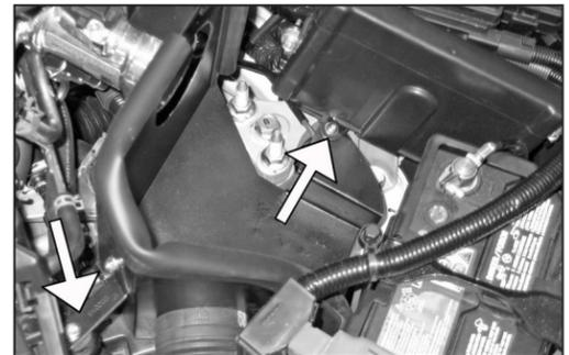
25. Attach the "L" bracket to the heat shield, and then install a bolt through the hole on the ECU bracket to the threaded boss on the heat shield. Then attach the factory air inlet hose to the heat shield.
