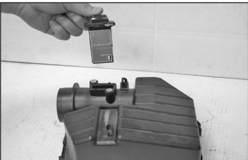
14. Loosen and remove the two screws that hold the MAF sensor to the factory airbox and remove the MAF sensor.
