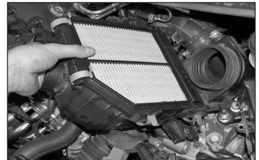
10. Pull up and twist downward to remove the lower factory airbox and intake tube.
