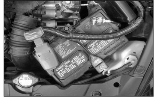
21. Loosen the positive battery cable and unclip the battery wire harness, adjust battery cable as shown. Then resecure the battery.
