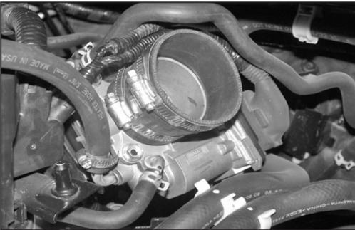
13. Install the silicone hose and hose clamps onto the throttle body as shown.
