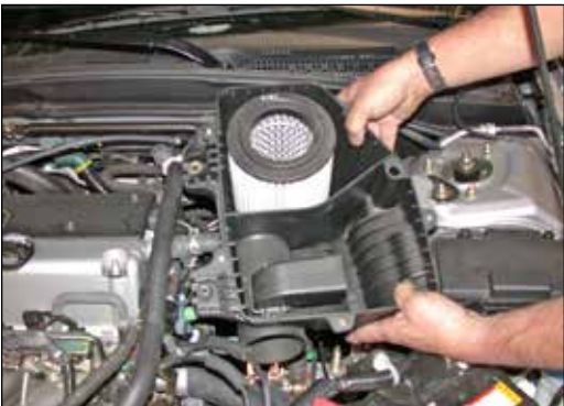
11. Pull upwards to remove the lower air cleaner assembly as shown.
