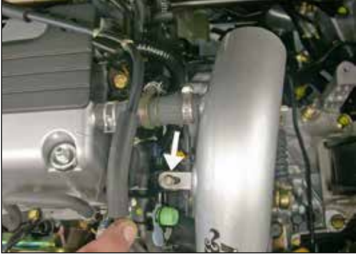
20. Using a 10mm socket secure the bracket to the air cleaner mounting point using the provided hardware.
