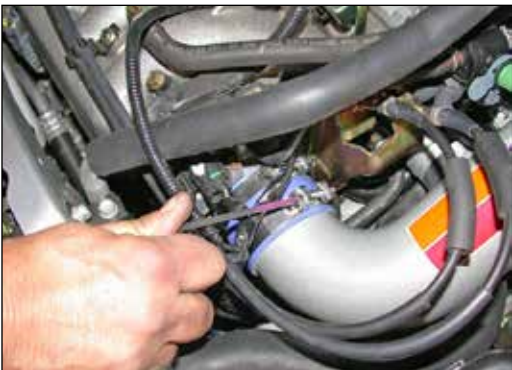
21. Using a flat blade screwdriver, tighten the hose clamp on the silicone hose as shown.
