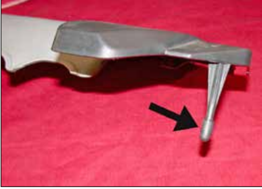
25. Install the rubber cap plug onto the stand off on the engine cover as shown.
