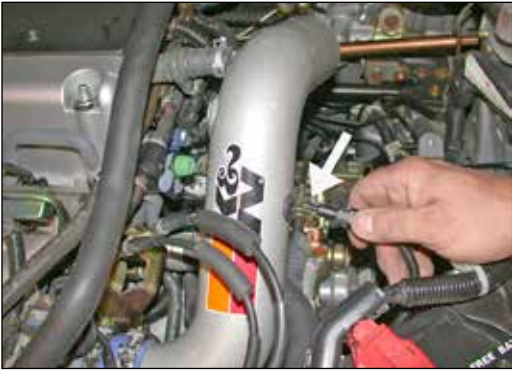
23. Push the air temperature sensor into the grommet on the K&N intake tube as shown.
