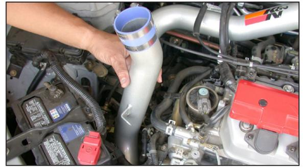
22. Install the tube as shown turning the tube in a clockwise rotation while inserting the tube in between the battery tray and the starter solenoid.
