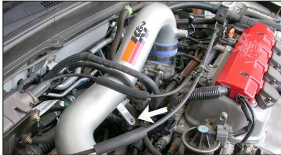
18. Install the K&N® intake tube onto the throttle body, then, line up the bracket with the rubber mounted stud as shown. Tighten hose clamps at this time.
