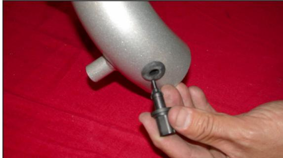
17. Install the provided rubber grommet into the hole on the K&N® intake tube, then install the air temperature sensor into the grommet as shown.
