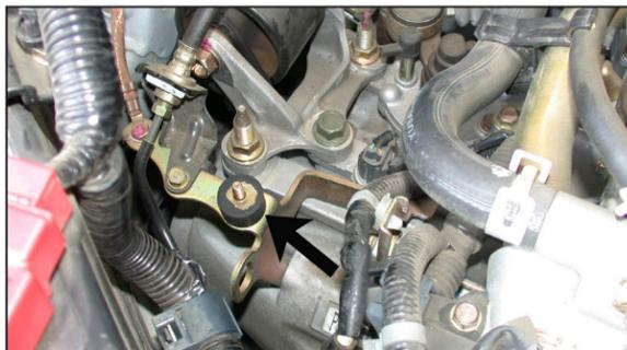
20. Install the remaining rubber mounted stud to the lower resonator mounting point as shown.
