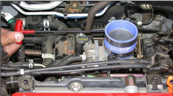
14. Install the silicone hose and hose clamps onto the throttle body. Do not tighten at this time.
