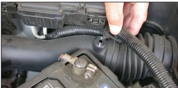
3. Unclip the battery cable from the air inlet duct as shown.
