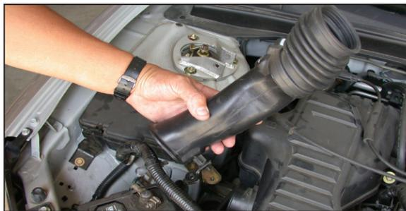
5. Remove the air inlet duct.
