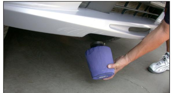
25. Raise the vehicle up and support it with jack stands, then, install the K&N® air filter from underneath the vehicle as shown.
