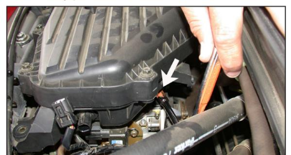
8. Loosen the hose clamp that secures the plenum to the throttle body as shown.
