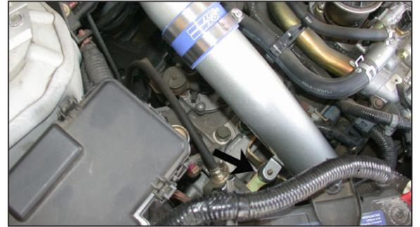
23. Slide the K&N® cold air tube onto the throttle body tube and line up the bracket with the rubber mounted stud as shown and secure with the provided hardware. Do not tighten completely.
