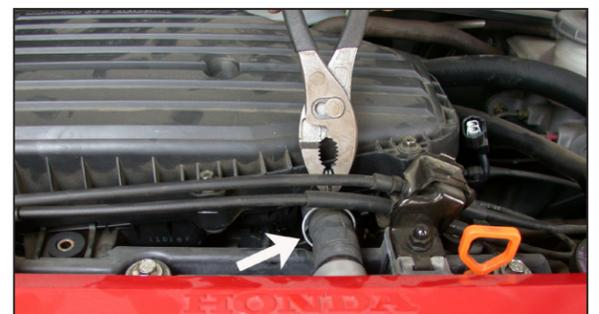
9. Using a pair of pliers, depress and pull back the hose clamp on the crank case vent at the cam cover.
