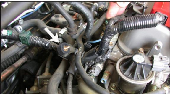
15. Install the rubber mounted stud onto the stock resonator mounting location as shown.
