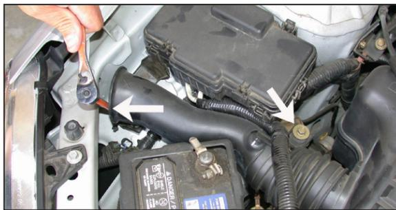
4. Loosen and remove the two bolts that secure the air inlet duct as shown.
