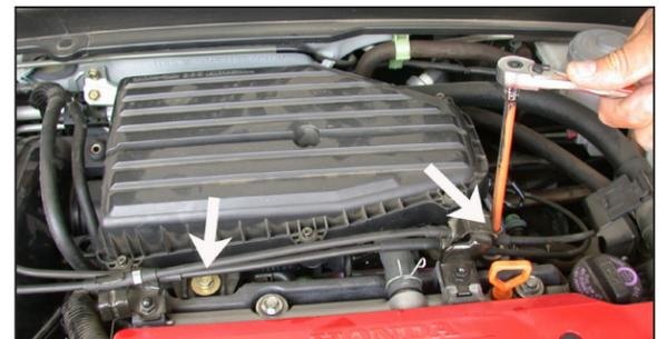
7. Loosen and remove the two bolts that secure the throttle body plenum.
