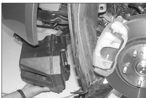
14. Remove the resonator as shown.
