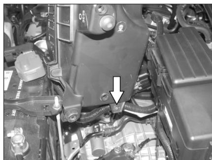
6. Lift the air cleaner assembly upwards, then, unclip the wire harness from the tab on the air cleaner assembly as shown.
