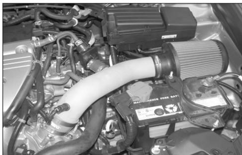
33. This K&N® high flow intake system has been designed to be used in two different configurations. In the case of inclement weather, the cold air tube can be removed and the air filter can be clamped onto the intake tube located in the engine compartment to avoid the possibility of ingesting water into the engine.
