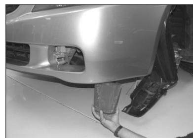
29. Install the filter from underneath the vehicle and secure it using the provided hose clamp.
