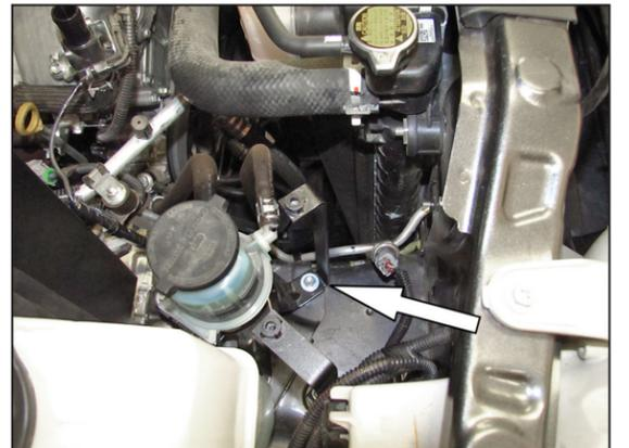
19. Install the provided secondary air pump mounting bracket (083168) onto the power steering reservoir using the bolt from the previous step.
