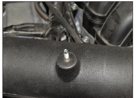
35. Install the engine cover mounting stud into the K&N® intake tube.
