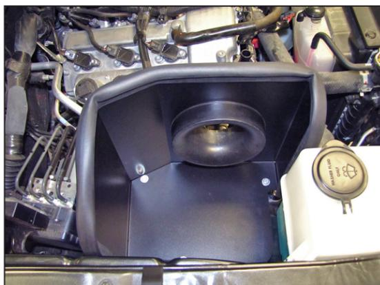
16. Set the heat shield into position on the rubber mounted studs and then secure with the provided hardware.
