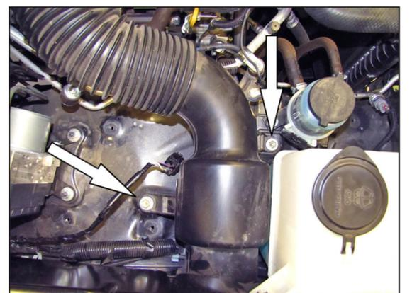
6. Remove the two bolts securing the intake resonator to the inner fender and then remove the intake tube/resonator assembly from the engine compartment.
