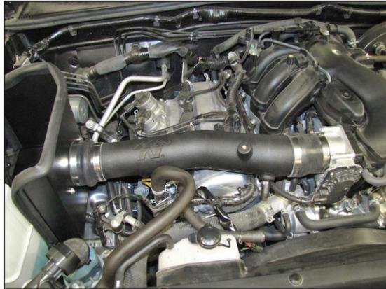
30. Install the K&N® intake tube into the silicone hose at the filter adapter far enough to gain clearance into the silicone hose at the throttle body, then install the tube into the throttle body silicone hose and secure with the provided hose clamps. **NOTE:** Do not completely tighten at this time.
