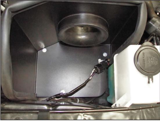
22. Route the secondary air wiring harness through the heat shield and reconnect the electrical connection.
