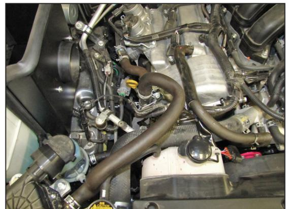
21. Install the secondary air pump onto the brackets previously installed and secure with the provided hardware. Reconnect the secondary air hose to the fitting and secure with the factory spring clamp.
