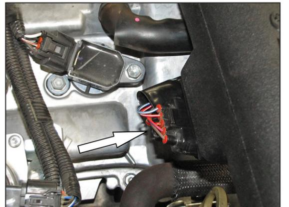
33. Reconnect the mass air sensor electrical connection.
