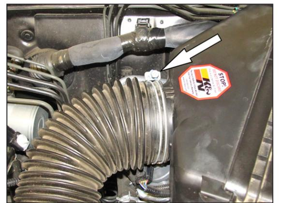
5. Loosen the hose clamp securing the intake tube to air filter housing.
