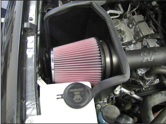
37. Install the K&N® air filter and secure with the provided hose clamp.
