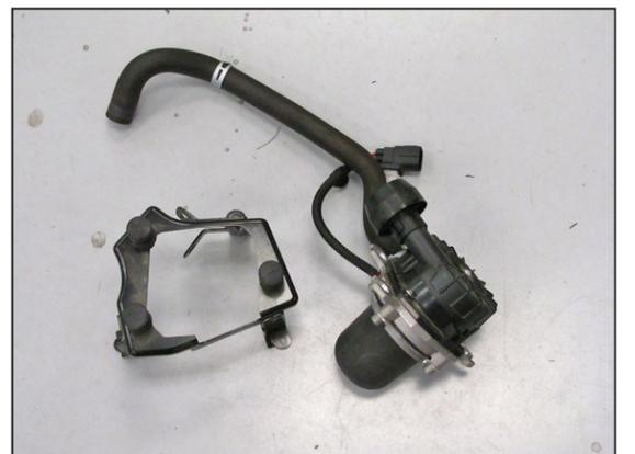
20. Separate the secondary air pump motor from the mounting bracket.
