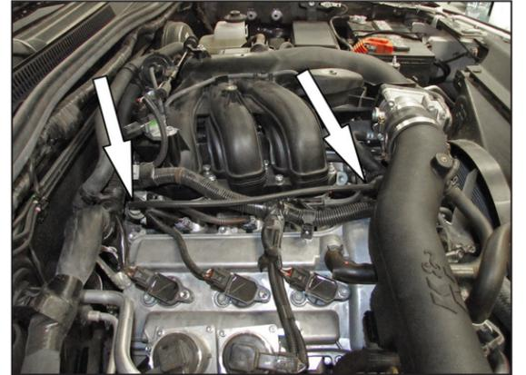
32. Connect the provided fuel pressure vent hose to the fuel pressure regulator and then connect the open end to the fitting installed into the K&N® intake tube.
