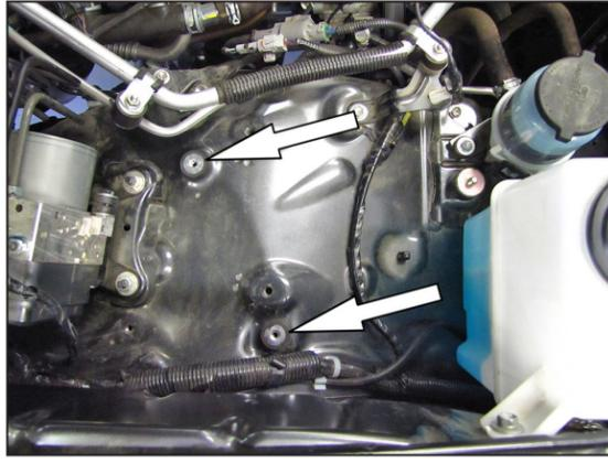
12. Install the two remaining 6mm rubber mounted studs into the secondary air injection pump mounting locations.
