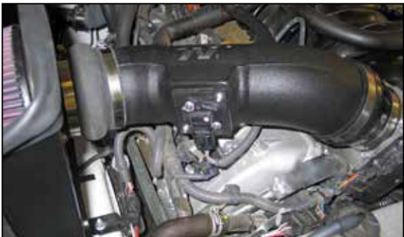
27. Reconnect the mass air sensor electrical connection.
