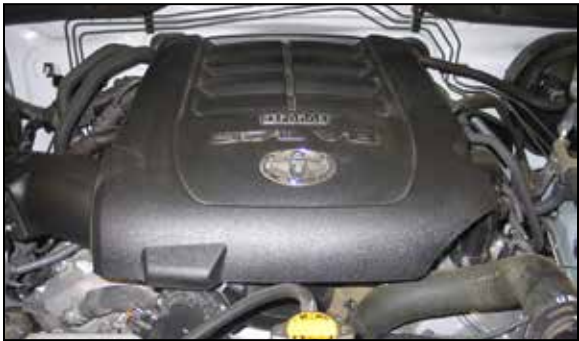
32. Install the engine cover.
