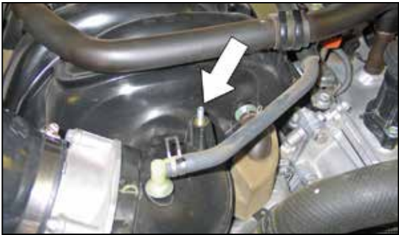
29. Install the provided stud into the mounting stud location as shown.
