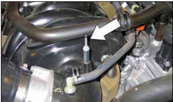
31. Install the factory mounting stud into the nut extension as shown.
