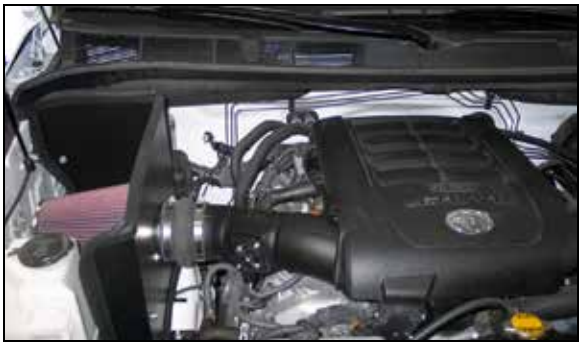
33. Reconnect the vehicle's negative battery cable. Double check to make sure everything is tight and properly positioned before starting the vehicle.
