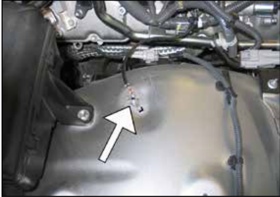
18. Remove the bolt that secures the ground strap to the inner fender. NOTE: This bolt will be reused.
