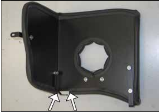
17. Install the provided longer edge trim onto the heat shield as shown. NOTE: Trimming of the edge trim will be necessary.
