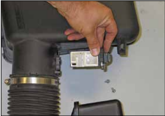
21. Remove the mass air sensor from the factory airbox.
