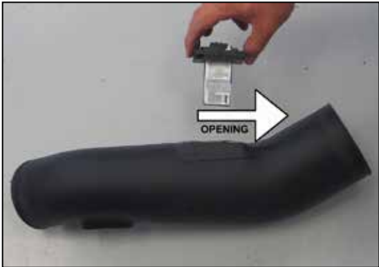
23. Install the mass air sensor assembly into the K&N® intake tube as shown using the provided hardware. NOTE: Ensure the opening is pointed towards the filter end of the intake tube.
