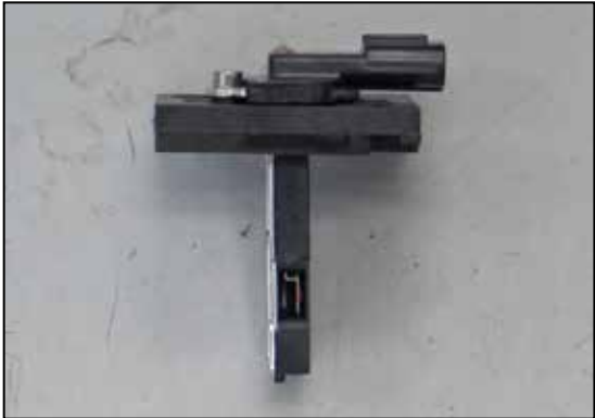
22. Install the mass air sensor into the K&N® mass air sensor adapter and secure with the provided hardware.
