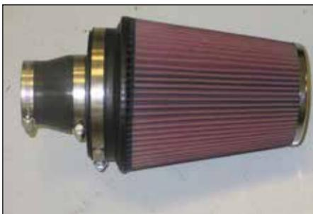
31. Install the provided silicone hose (084055) onto the filter adapter and secure with the provided hose clamp.
