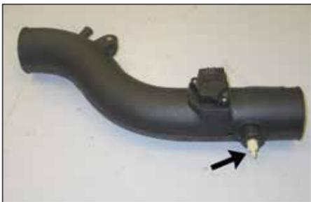
26. Install the 1/4" npt fitting into the K&N® Intake Tube as shown.
