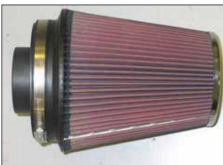
30. Install the filter adapter into the K&N® Air Filter and secure with the provided hose clamp.
