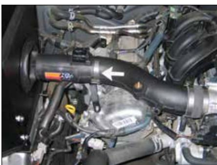
28. Install the K&N® Intake Tube assembly into the silicone hose at the throttle body and align with the tube mounting bracket assembly, then secure with the provided hose clamps.
