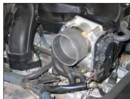
22. Install the provided silicone hose (08711) onto the throttle body and secure with the provided hardware.
