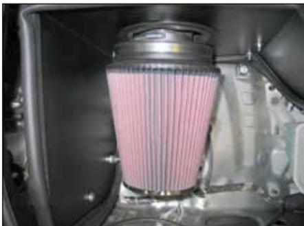
32. Install the filter assembly onto the K&N® Intake Tube and secure with the provided hose clamp.
