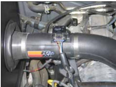
34. Reconnect the Mass air sensor electrical connection.
