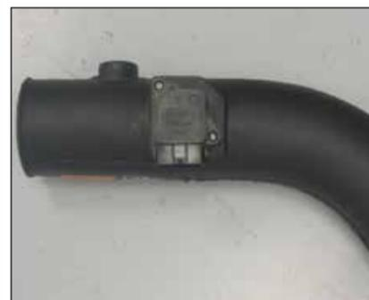
25. Install the mass air sensor into the K&N® Intake Tube and secure with the provided bolts and spacers.
