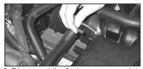
5. Disconnect the fuel pressure regulator vent hose from the factory intake tube as shown.
