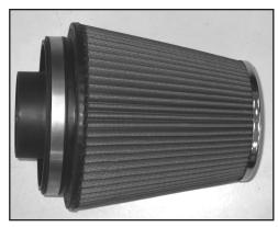
29. Install the air filter adapter into the K&N<sup>®</sup> air filter and secure with the provided hose clamp as shown.
