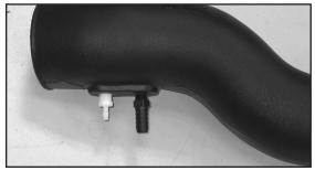
23. Install the provided NPT fittings into the intake tube in the positions shown.
