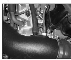
28. Connect the hose mender from the crank case vent hose assembly into the factory crank case vent hose and secure with the factory spring clamp. Then, connect the open end to the intake tube as shown.
