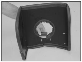
10. Install the small edge trim into the hole of the heat shield as shown.
