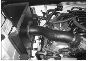
25. Install the intake tube into the silicone hose at the throttle body and align with the the bracket installed on the heat shield. Align tube and heat shield then tighten the heat shield and secure the intake tube with the provided hardware.
