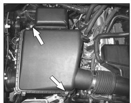
7. Loosen the two bolts that secure the air box to the inner fender.
