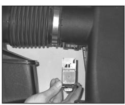
20. Remove the two bolts that secure the mass air sensor into the stock air filter housing. Remove the mass air sensor as shown.
