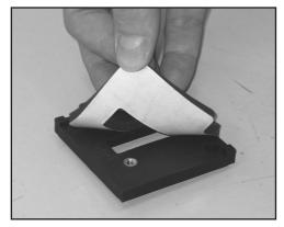
19. Install the provided gasket onto the mass air sensor adapter as shown.
