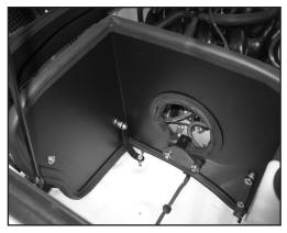
17. Secure the rear lower mounting bracket to the ground strap location with the provided hardware.
