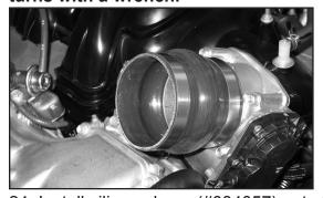
24. Install silicone hose (#084057) onto the throttle body and secure with the provided hose clamp as shown.
