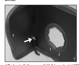
12. Install the small "L" bracket (#07190) onto the heat shield with the provided hardware and spacers as shown.
