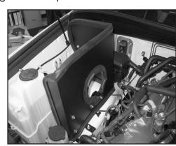
16. Set the heat shield into position on the inner fender. Then, secure the front mounting bracket to the front air box mounting location with the provided hardware.
