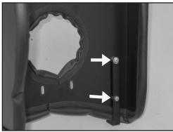
11. Install the large "L" bracket (#070902) onto the heat shield using the provided hardware and spacers as shown.
