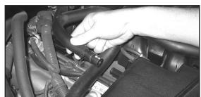
4. Disconnect the crank case vent hose from the factory intake tube as shown.
