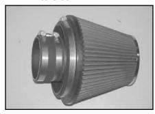
22. Install the silicone hose (08630) onto the K&N<sup>®</sup> Air filter assembly and secure with the provided hose clamp.
