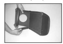
10. Install the edge trim onto the heat shield as shown. Trim if needed.
