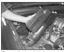
7. Remove the three bolts that retain the air box to vehicle, then remove the air box.
