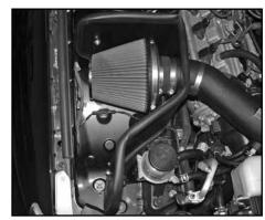
23. Install the K&N® Air filter onto the intake tube as shown and secure with the provided hose clamp.
