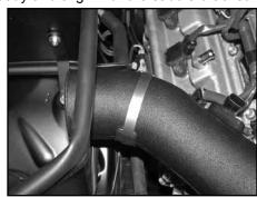
19. Secure the K&N® intake tube to the saddle bracket with the provided hose clamps also tighten the hose clamp at the throttle body.
