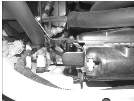
17. Secure the heat shield bracket to the radiator fan shroud with the bolt removed in step #15.
