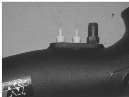
19. Install the provided npt fittings into the intake tube as shown.
