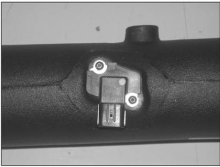
10. Install the mass air sensor into the K&N® intake tube and secure with the provided spacers and hardware as shown.
