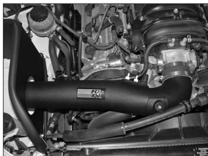
20. Install the intake tube onto the throttle body and align with the tube mounting bracket, Then secure with the provided hardware.
