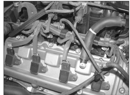
22. Remove the factory crankcase vent hose and fuel pressure regulator vent hose shown from the engine.
