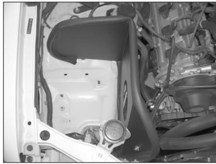
16. Install the heat shield assembly onto the rubber mounted studs install in step #14 and secure with the provided hardware.
