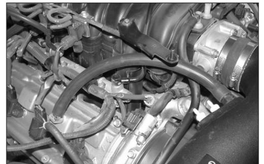
23. Install the provided crankcase vent hose onto the valve cover and then attach to the intake tube as shown.
