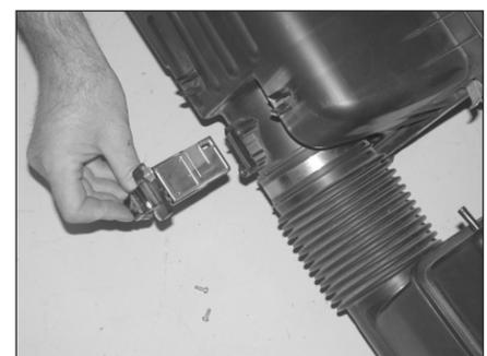
9. Remove the two screws which secures the mass air sensor to the factory airbox, then remove the mass air sensor from the airbox as shown.
