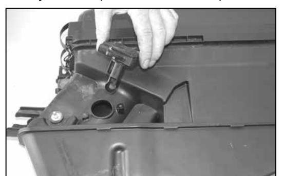
21. Remove the two screws that secure the mass air sensor to the air box assembly, then remove the mass air sensor as shown.
