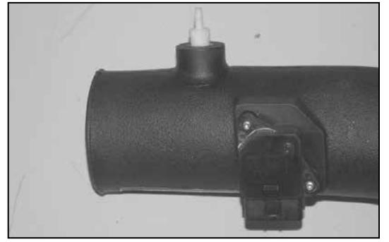
24. Install the vent fitting into the K&N® intake tube as shown.
