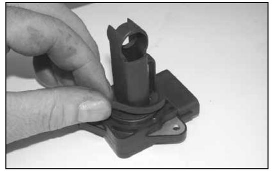
22. Apply the gasket to the mass air sensor, sticky side down as shown.
