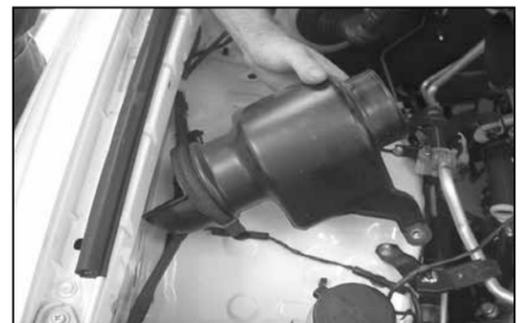
6. Remove the two bolts that secure the resonator to the inner fender, then remove the resonator from the vehicle as shown.
