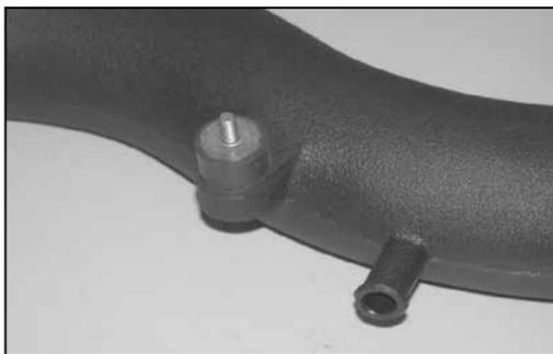
25. Install the rubber mounted stud onto the K&N® intake tube as shown.
