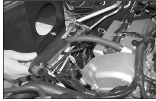
17. Remove the factory crank case vent hose from the valve cover, reverse the hose and reconnect onto the valve cover as shown.
