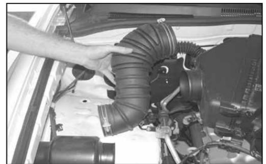
5. Remove intake tube from the vehicle as shown.
