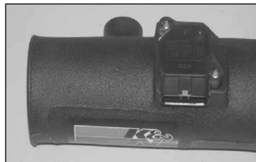
23. Secure the mass air sensor to the K&N® intake tube using the provided screws and spacers as shown.
