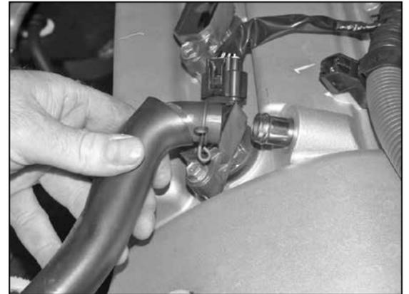
19. Remove crank case vent hose from valve cover.
