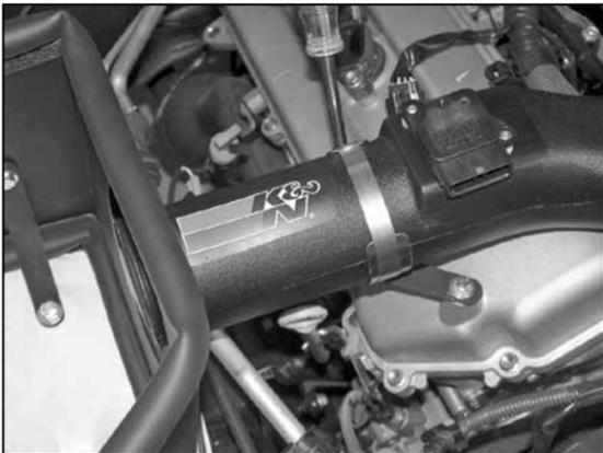
28. Secure the K&N® intake tube to the saddle bracket with the provided hose clamps also tighten the hose clamp at the the throttle body.
