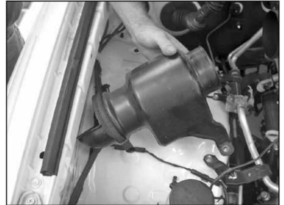
6. Remove two bolts that secure resonator to inner fender, then remove resonator from vehicle as shown.
