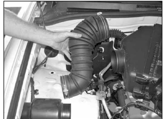
5. Remove intake tube from vehicle as shown.
