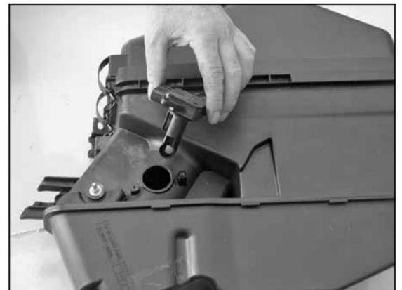
22. Remove the two screws that secure the mass air sensor to the air box assembly, then remove the mass air sensor as shown.
