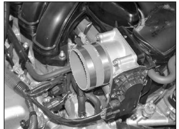
21. Install the provided silicone hose (08434) onto throttle body with the provided hose clamp as shown.
