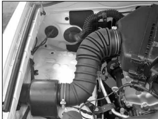
3. Loosen the hose clamps at the air box and resonator.
