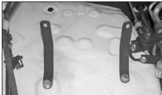
15. Mount the two provided brackets onto the vehicle with the provided hardware.
