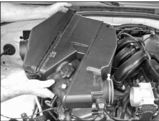
11. Remove air box assembly from engine as shown.
