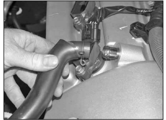
19. Remove crank case vent hose from valve cover.
