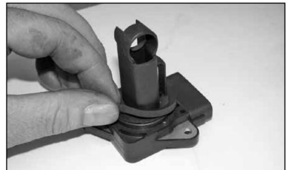
23. Apply the gasket to the mass air sensor, sticky side down as shown.
