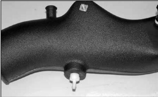
25. Install the vent fitting onto the K&N® intake tube as shown.
