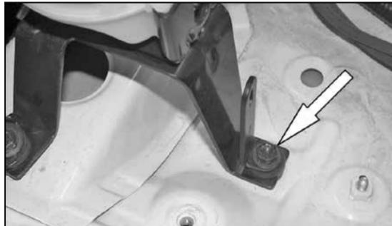
14. Remove the 12mm bolt that retains the power steering reserve to vehicle, then mount the provided bracket (07158) onto the vehicle with the bolt that was removed.
