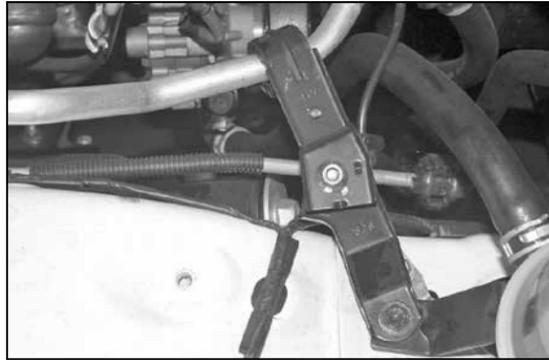
13. Rotate the A/C mounting bracket onto the power steering reservoir, then secure it using the bolt from the previous step. Tighten the A/C mounting nut.
