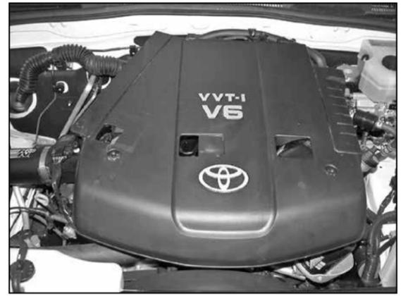
33. Re-install the engine cover using the original nuts removed in step #1.
