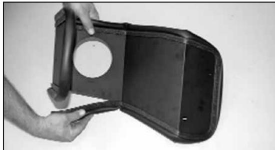
16. Install the edge trim onto the heat shield as shown. Trim if needed.
