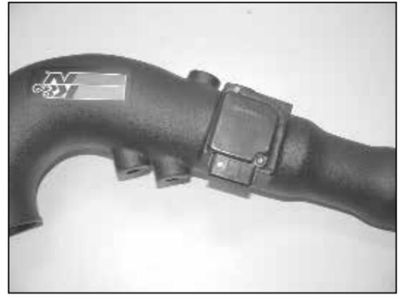
17. Secure the mass air sensor to the K&N® intake tube using the provided screws and spacers as shown.
