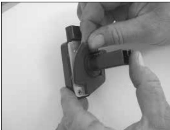
16. Apply the gasket to the mass air sensor, sticky side down as shown.
