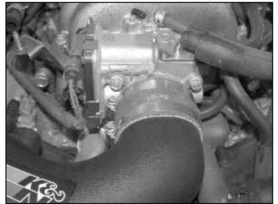
19. Install the K&N® intake tube onto the throttle body and align with the saddle bracket.
