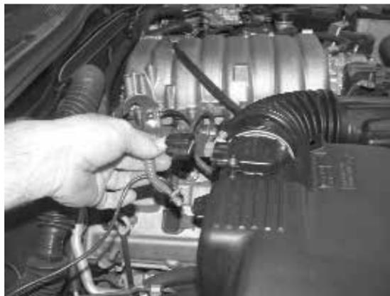
3. Disconnect the mass air sensor electrical connection, then release wire loom from air box.
