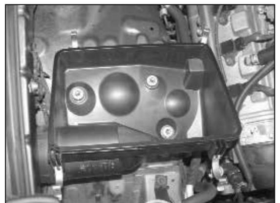
6. Remove the air box lid and filter to gain access to the three bolts that retain the air box to vehicle.
