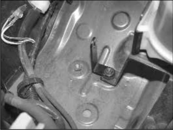
8. Remove the 12mm bolt that retains the power steering reserve to vehicle then mount the provided bracket (070632) onto the vehicle with the bolt that was removed.
