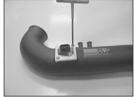
23. Secure the mass air sensor assembly onto the K&N® intake tube with the provided hardware.
