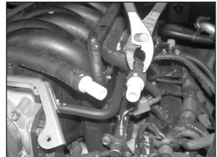
26. Install the provided hose mender into the two crank case vent hoses and secure the existing spring clamps as shown.
