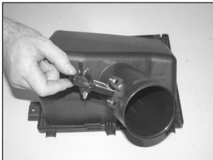
19. Remove the two screws that secure the mass air sensor to the air box lid, then remove the mass air sensor as shown.
