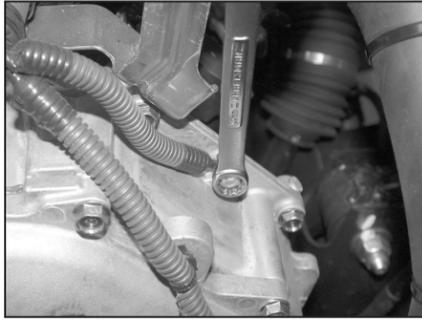
16. Locate the ground wire attached to the engine cam cover and remove the bolt securing it using a 10mm wrench.
