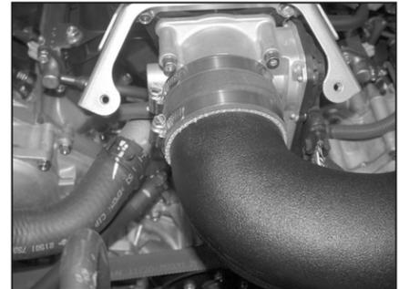
24. Install the K&N® intake tube onto the throttle body and align with the saddle bracket.
