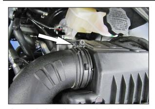
7. Loosen the hose clamp securing the intake tube to the air filter housing and then remove the intake tube from the vehicle.
