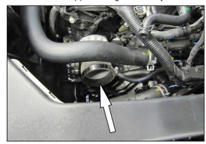
19. Install the provided coupling hose (08711) onto the throttle body and secure with the provided hose clamp.
