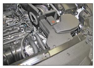
18. Install the fresh air intake scoop into the heat shield and onto the core support. Secure the scoop to the heat shield using the panel and hardware and to the core support using the factory retainers.
