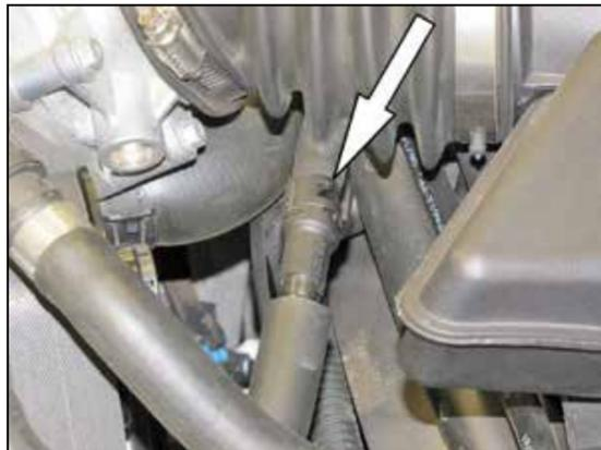
4. Disconnect the crank case vent tube from intake tube.
