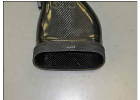
7. Slide the silicone hose (08619) onto the K&N® intake tube so that only approximately 1/4" of the hose is not installed.
