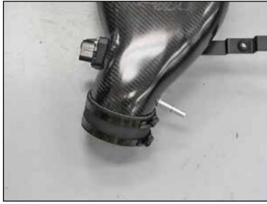
14. Install the provided silicone hose (08761) onto the K&N® intake tube but do not tighten the hose clamps at this time.
