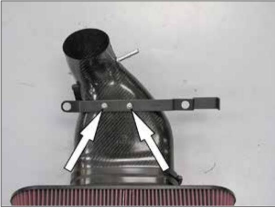
10. Install the tube mounting bracket onto the K&N® intake tube using the provided hardware.
