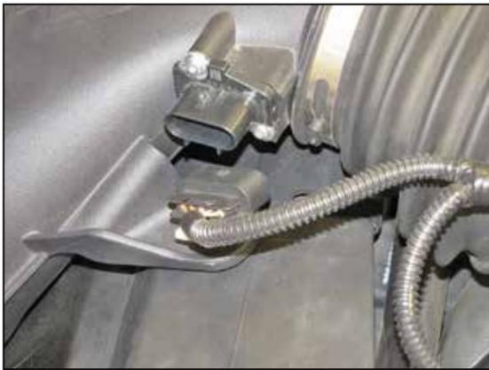
2. Disconnect the mass air sensor electrical connection and unclip the wiring harness from the intake tube.
