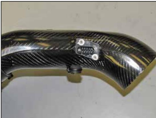
13. Install the mass air sensor into the K&N® intake tube and secure with the provided hardware.
