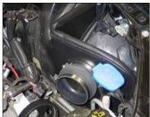
15. Install the provided silicone hose (08418) onto the filter adapter and secure with the provided hose clamp.
