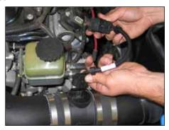
22. Connect the provided mass air sensor extension harness to the factory connector and then to the mass air sensor as shown. Route the wiring harness behind the mass air sensor for clearance from the engine cover.
