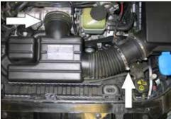
4. Loosen the two hose clamps which secure the stock intake tube to the throttle body and mass air sensor.
