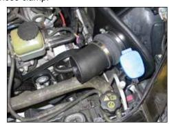
18. Install the small intake tube into the silicone hose at the filter adapter as shown.
