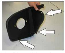
11. Install the provided edge trim onto the heat shield as shown.
