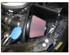
$25. \ \mbox{Install}$  the air filter and secure with the provided hose clamp.
