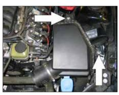
7. Remove the two air box mounting nuts shown.
