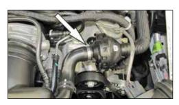
3A. On vehicles equipped with a sound drum, disconnect the sound tube from the drum and cap off the drum with the provided caplug.
