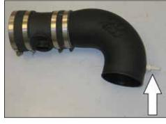
20. Install the crankcase fitting into the K&N<sup>®</sup> intake tube as shown.
