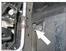
9. Remove the air box mounting stud shown.
