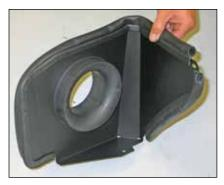
12. Install the filter adapter into the heat shield and secure with the provided hardware.
