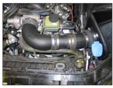
21. Install the K&N® intake tube with mass air sensor into the silicone hose at the throttle body and onto the intake tube on the filter adapter. Rotate and adjust the intake tubes for proper fit and then secure the assembly with the hose clamps.
