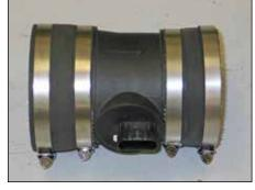
17. Install the provided silicone hose (08536) onto the mass air sensor and secure with the provided hose clamp.
