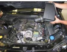
8. Remove the complete air box assembly from the vehicle.
