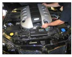
2. Remove the oil fill cap and then remove the engine cover from the engine as shown. Reinstall the oil fill cap.
