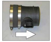
16. Loosen the hose clamp and remove the mass air sensor from the factory air box. Install the provided silicone hose (08761) onto the mass air sensor and secure with the provided hose clamp.
