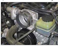
14. Install the silicone hose (08618) onto the throttle body and secure with the provided hose clamp.
