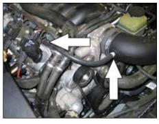
23. Connect the crank case vent hose to the valve cover port and then connect the open end to the vent fitting installed into the K&N® intake tube.
