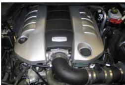
24. Remove the oil fill cap and reinstall the engine cover. Reinstall the oil fill cap.
