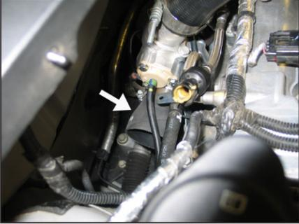
10. Install the provided silicone hose (08713) onto the turbo inlet and secure with the provided hose clamp.
