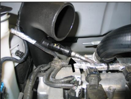
13. Connect the crank case vent hose to the quick connect fitting.
