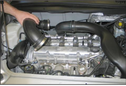
9. Loosen the hose clamp which secures the stock intake tube to the turbo inlet and then remove the intake tube from the vehicle.
