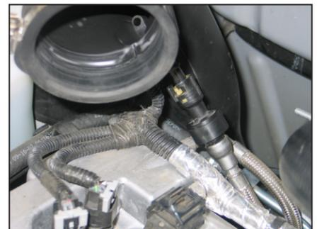
8. Release the crank case vent tube from the fitting on the stock intake tube.
