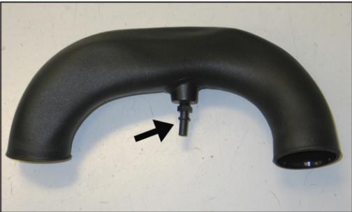
11. Install the provided crank case quick connect fitting into the K&N® intake tube as shown.
