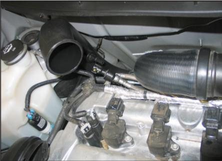
12. Install the K&N® intake tube into the silicone hose at the turbo inlet and secure with the provided hose clamp.
