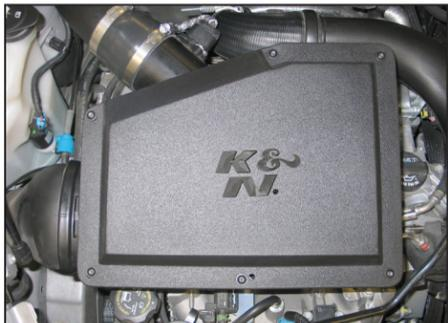
18. Install the K&N® air box lid and secure with the six factory screws.
