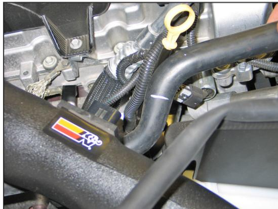
18. Mark the air injection hose at the base of the top 90deg bend as shown.
