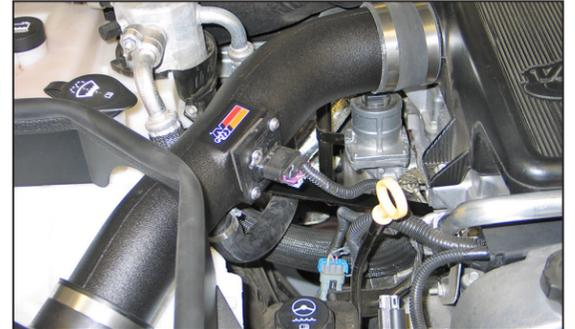
21. Reconnect the mass air sensor electrical connection as shown.
