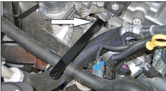
12. Install the tube mounting bracket (26632) onto the engine at the ground cable location and secure with the bolt removed in step #11.
