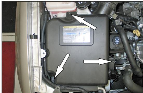
4. Loosen the three screws which secure the upper air box.
