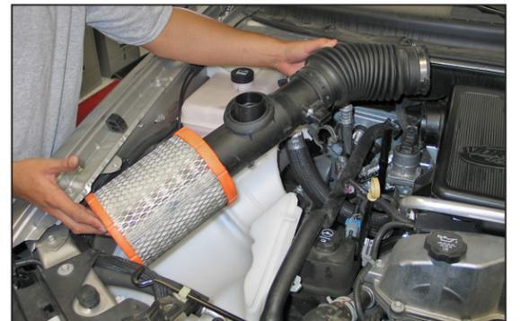
7. Loosen the hose clamp at the intake plenum and then remove the complete intake system.
