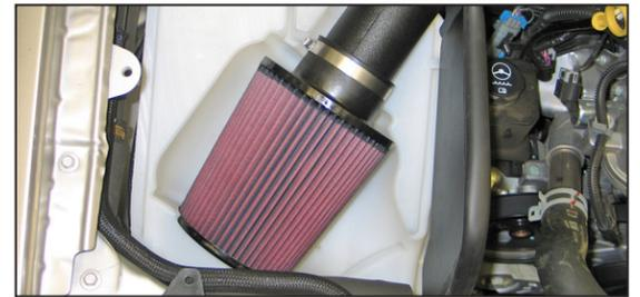
20. Install the K&N air filter onto the K&N intake tube and secure with the provided hose clamp. **NOTE: Drycharger air filter wrap; part # RX-4730DK is available to purchase separately. To learn more about Drycharger filter wraps or look up color availability please visit <http://www.knfilters.com>.**
