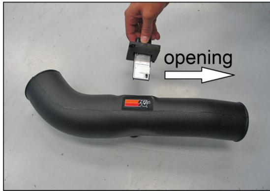
16. Install the mass air sensor assembly into the K&N intake tube and secure with the provided hardware.
