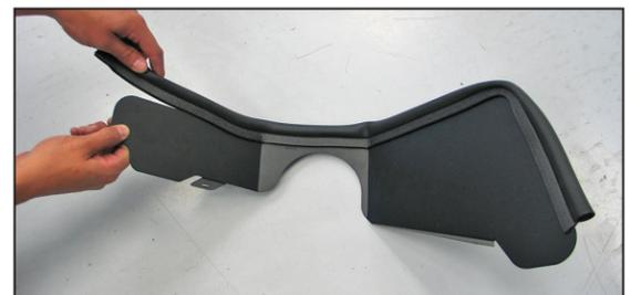
9. Install the provided edge trim onto the heat shield as shown.
