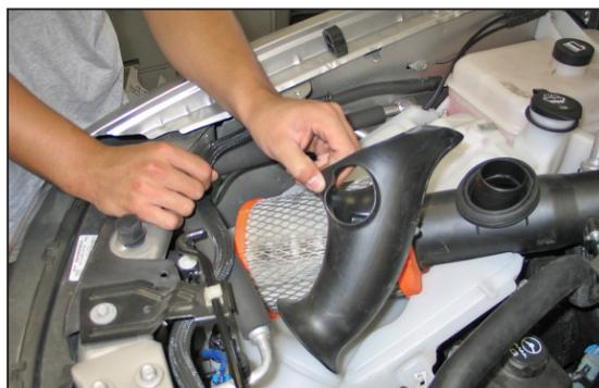
6. Remove the fresh air supply duct.
