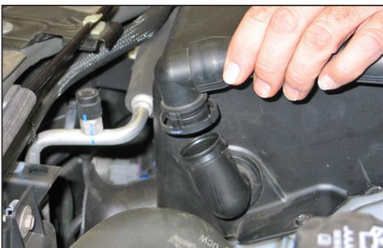
3. Depress the locking tabs and disconnect the air injection hose.
