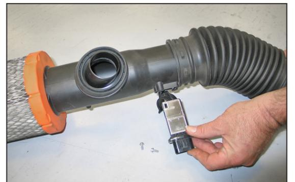
8. Remove the two screws which secure the mass air sensor. Then remove the mass air sensor as shown.
