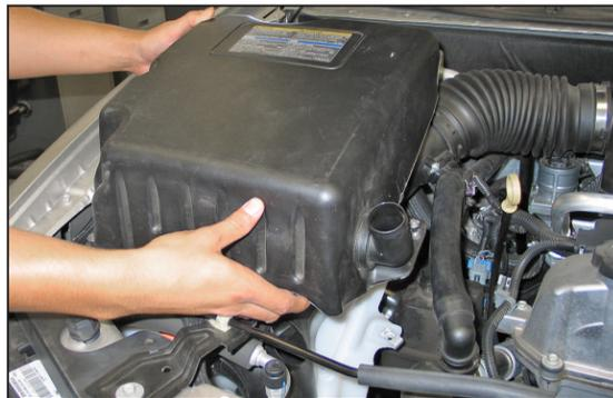
5. Remove the upper air box cover as shown.
