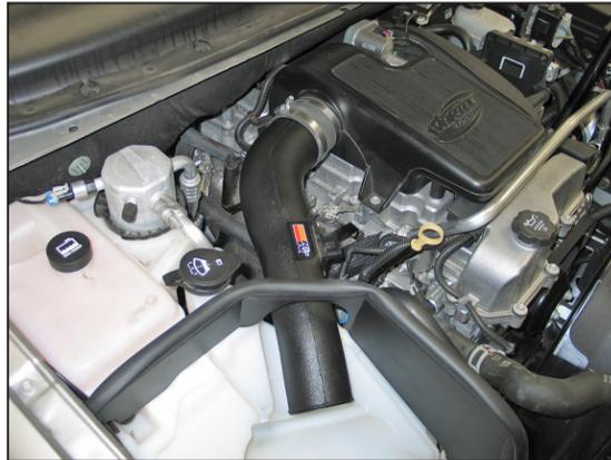
17. Install the K&N intake tube assembly into the silicone hose at the throttle body and align it with the mounting bracket installed in step #12. Then secure the tube with the provided hose clamp and hardware.
