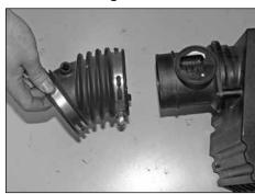
21. Loosen the hose clamp, which secures the stock intake tube to the mass air sensor, and then remove the hose from the sensor as shown.
