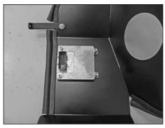
30. Secure the transmission control module to the heat shield with the provided hardware as shown. NOTE: Four washers should be placed between the heat shield and module to form an air gap.
