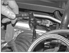
3. Release the locking tab and disconnect the crank case vent tube as shown.
