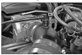
40. Reconnect the crank case vent tube to the vent fitting as shown.
