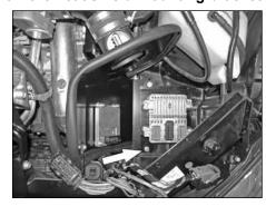
34. Place the engine control module assembly into position on top of the heat shield, then secure the heat shield and control module bracket to the inserted nuts installed in step #31 with the provided hardware.
