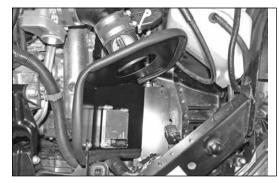
33. Install the heat shield assembly onto the inner fender and secure the mounting bracket to the radiator mount using the factory bolt removed in step #32.
