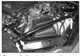
6. Remove the three body support brace mounting bolts shown and then remove the support brace from the engine compartment.
