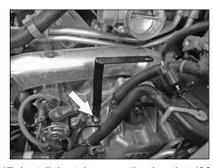
17. Install the tube mounting bracket (26627) onto the existing transmission stud as shown.
