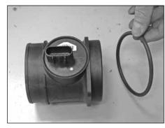
23. Remove the "O" ring from the mass air sensor as shown.
