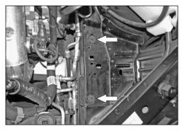
31. Install the two inserted nuts into the air box mounting grommet holes as shown.
