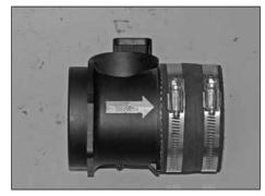
26. Install the silicone hose (08690) onto the mass air sensor as shown and secure with the provided hose clamps.
