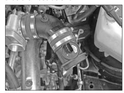
27. Install the mass air sensor assembly onto the K&N® intake tube as shown and secure with the provided hose clamp.
