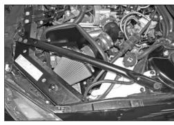
39. Reinstall the body brace removed in step #6 and secure with the factory bolts.
