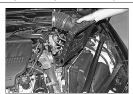
5. Remove the air box housing half and intake tube as shown.
