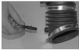
20. Remove the crank case vent fitting from the stock intake tube as shown.
