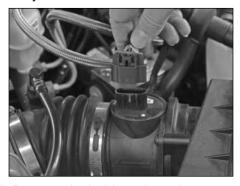
2. Depress the locking tab on the mass air sensor electrical connection, then disconnect the mass air sensor electrical connection as shown.
