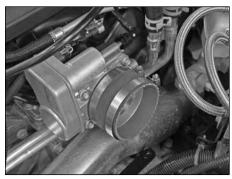
18. Install the silicone hose (08690) onto the throttle body and secure with the provided hose clamp.
