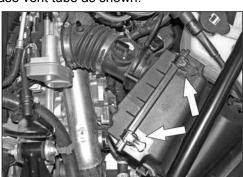
4. Loosen the hose clamp, which secures the intake tube to the throttle body, and release the air box over center clips shown.
