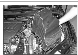
8. Remove the upper air box housing from the vehicle as shown.
