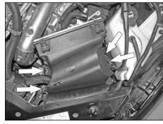
7. Depress the four air box housing retaining clips shown.
