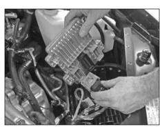
11. Release the engine control module wiring harness clamshell clips and disconnect the wiring harness from the engine control module.
