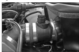
41. Reconnect the mass air sensor electrical connection.
