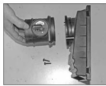
22. Remove the two screws, which secure the mass air sensor to the air filter housing and then remove the mass air sensor as shown.
