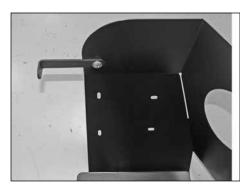
28. Install the mounting bracket (070952) onto the heat shield with the provided hardware.
