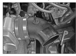
25. Install the K&N® intake tube into the silicone hose at the throttle body and align with the mounting bracket installed in step #17. Secure the silicone hose onto the throttle body with the supplied hardware and hose clamp.
