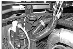
32. Remove the top left radiator mounting bracket bolt shown.
