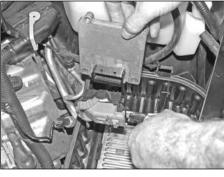
9. Remove the transmission control module from the housing, release the clamshell retaining clip, and then disconnect the wiring harness as shown.
