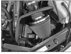
38. Install the air filter assembly onto the mass air sensor and secure with the provided hose clamp.
