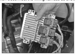
10. Release the engine control module from the mounting clip and lift the module from the base as shown.
