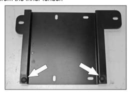
14. Install the rubber bumpers provided into the engine control module-mounting bracket (26628-1) as shown.
