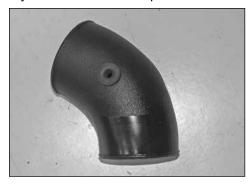
19. Install the provided grommet into the K&N<sup>®</sup> intake tube as shown.
