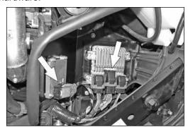
35. Reconnect the engine control module and transmission control module electrical connections.
