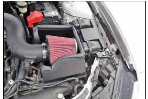
18. Install K&N filter onto K&N intake tube. Secure with provided hose clamp.
