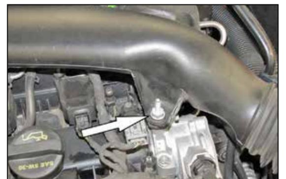
5. Loosen and remove the bolt that secures the intake tube to the engine.
