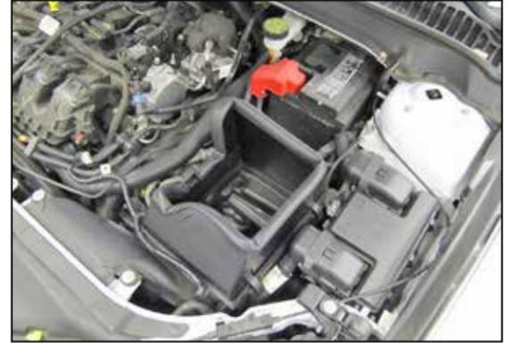
16. Install heat shield onto factory lower air box. Snap in place using factory retaining clips.
