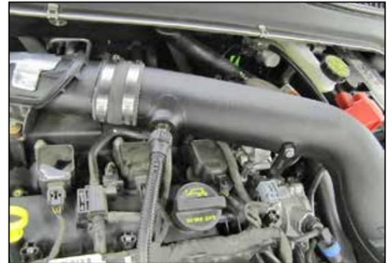
19. Connect crankcase vent line onto quick connect fitting on K&N intake tube.
