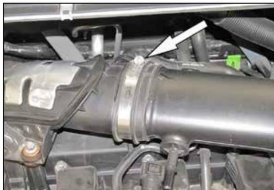
4. Loosen the hose clamp that secures the intake tube to the turbo inlet.
