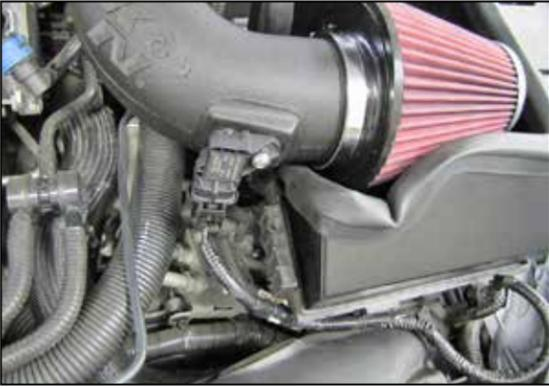
20. Reconnect pressure sensor electrical connector onto sensor.
