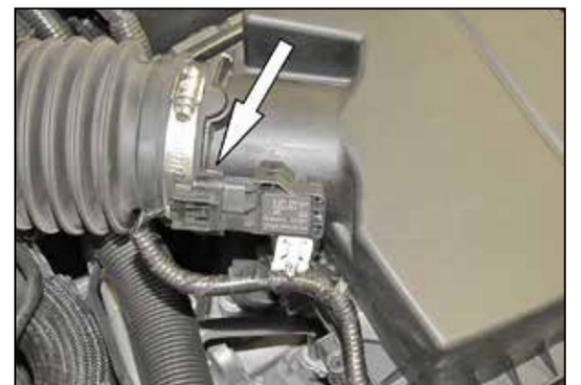
6. Disconnect the temperature sensor electrical connect.
