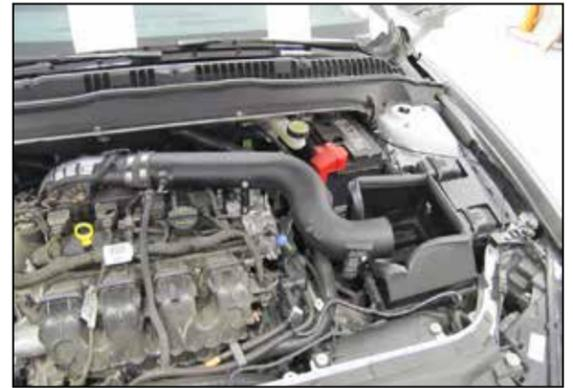
17. Install K&N intake tube into the hose and onto the tube mounting bracket. Align with heat shield and secure with provided hardware.
