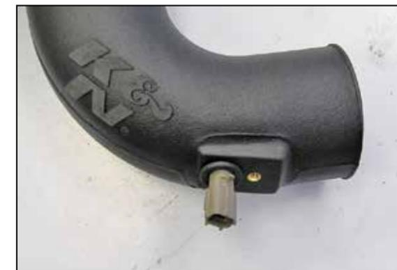
13. Install the temperature sensor into the K&N intake tube and secure with the provided hardware.
