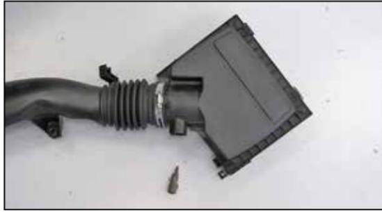
11. Remove the temperature sensor from the factory air box and then remove the "O" ring from the sensor.
