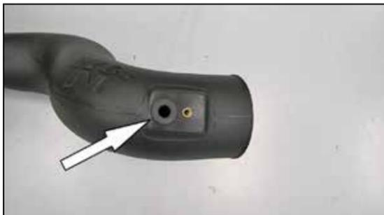
12. Install provided grommet into K&N intake tube.
