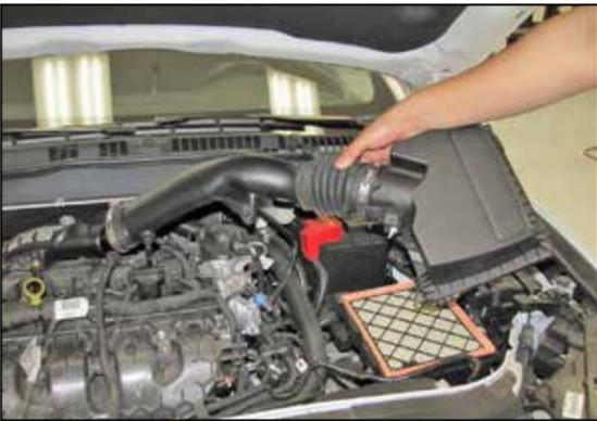
8. Release the two upper air box retaining clips and then remove the complete intake assembly.
